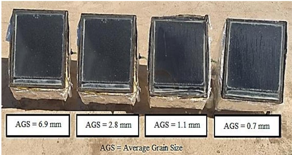
Figure 2. Image of the SSs used in the experiment
