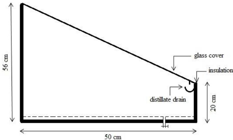
Figure 1. Schematic diagram of the fabricated solar stills
