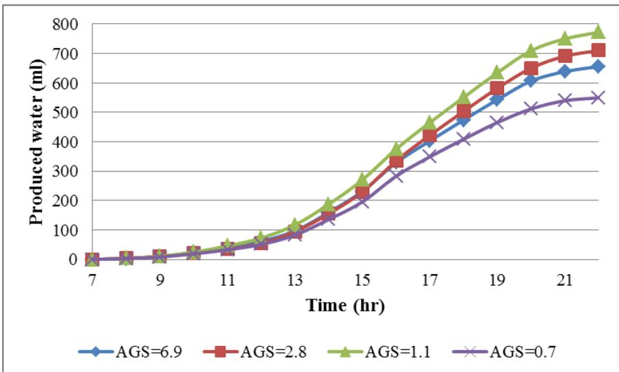
Figure 8. Cumulative water production of the stills
