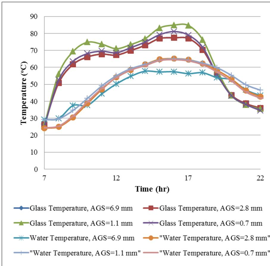
Figure 6. Changes in air temperature (under the glass cover) and water temperature inside the stills
