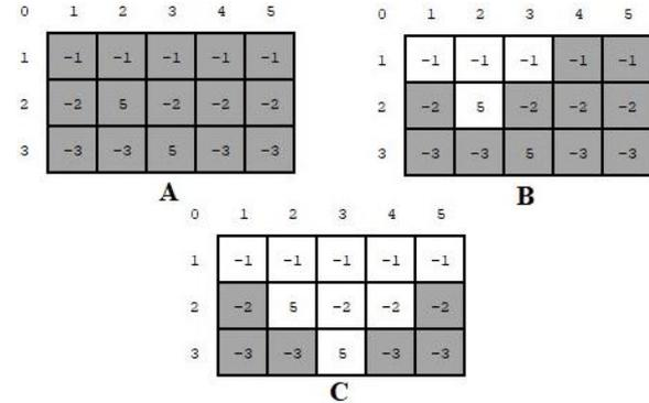
Figure 4: Formation of a larger cone with lower profit by floating cone algorithm
