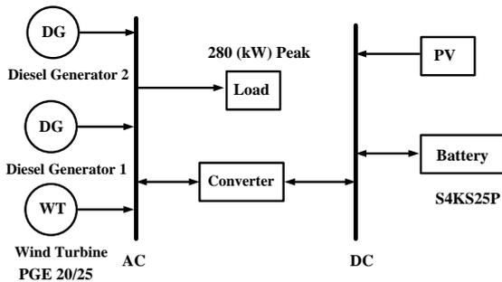
Figure 3. Detailed model of PV-wind -diesel-battery system
