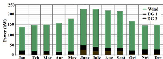
Figure 6. Monthly average power production of HRES installed in Zabol considering long-term wind speed changes
