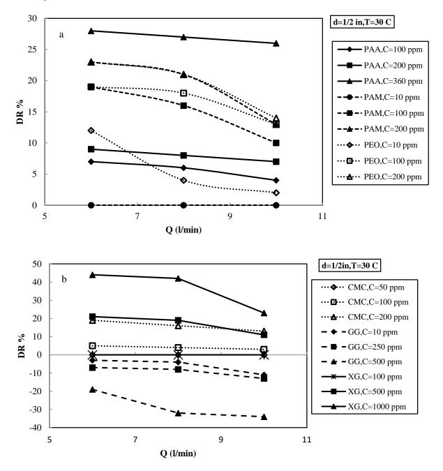
Fig. 4. The variation of the DR% with volume flow rate at different concentrations at d=1/2 in(a) Synthetic DRA (b) Biological DRA
