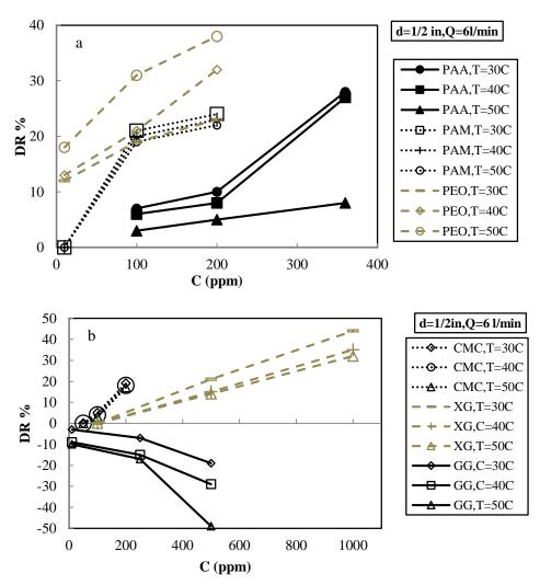
Fig. 6. The change in the DR% with concentration at various temperatures (d=1/2 in, Q=6 l/min), (a) Synthetic DRA (b) Biological DRA
