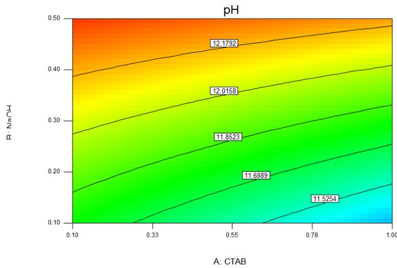
**Fig. 5.** Contour graph between the pH vs CTAB and NaOH concentration
