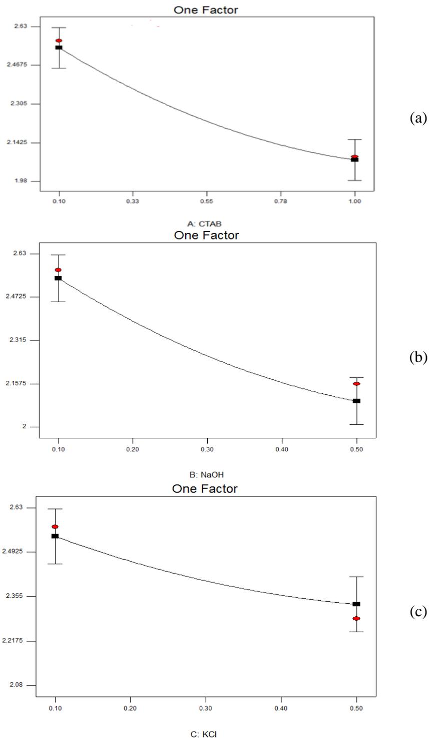
**Fig. 1.** Representation of single factor viscosity (cP) effect of (a) CTAB, (b) NaOH, and (c) KCL
