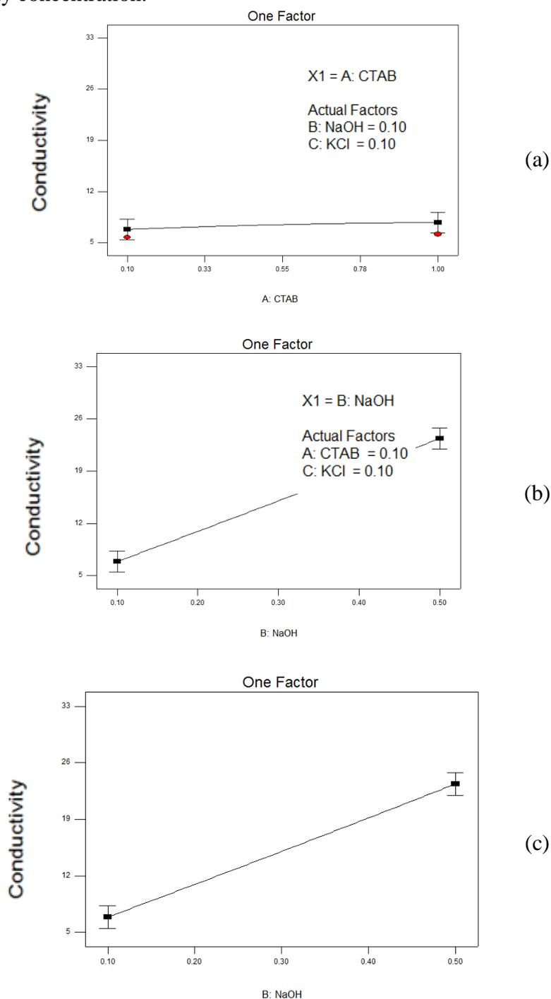
**Fig. 7.** Representation of single factor conductivity (mS/cm) effect of (a) CTAB, (b) NaOH and (c) KCl.
