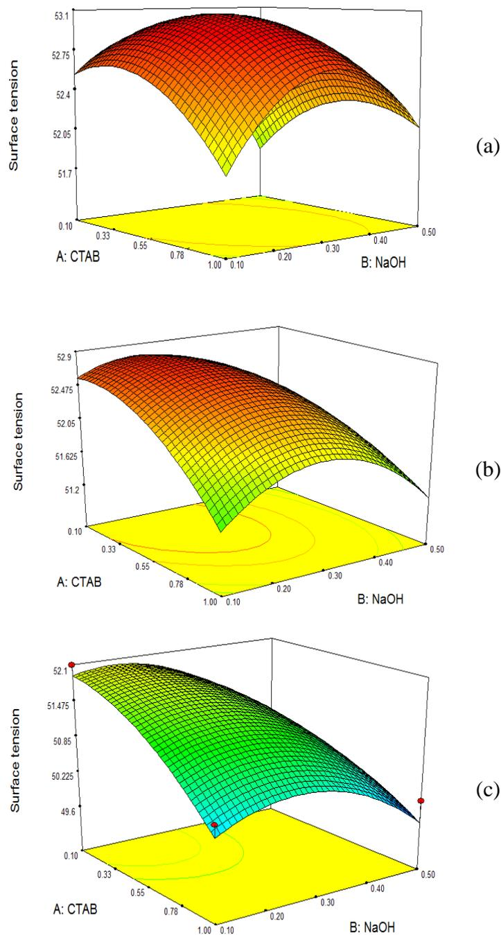
**Fig. 3.** Response surface plot for Surface Tension (dyne/cm) of CTAB and NaOH at (a) 0.10 wt% of KCl, (b) 0.20 wt% of KCl, (c) 0.30 wt% of KCl
