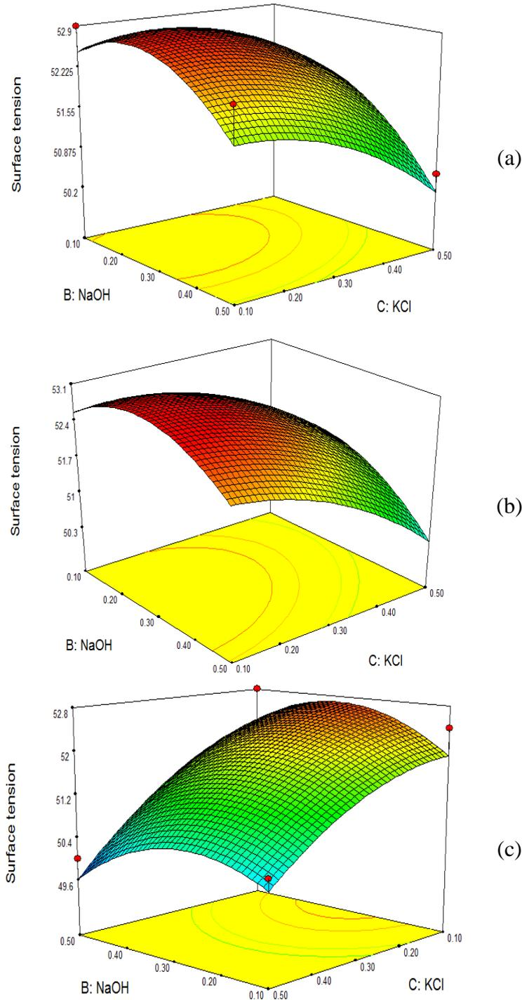
**Fig. 4.** Response surface plot for surface tension (dyne/cm) of NaOH and KCl at (a) 0.10 wt% of CTAB, (b) 0.50 wt% of CTAB, (c) 1.0 wt.% of CTAB
