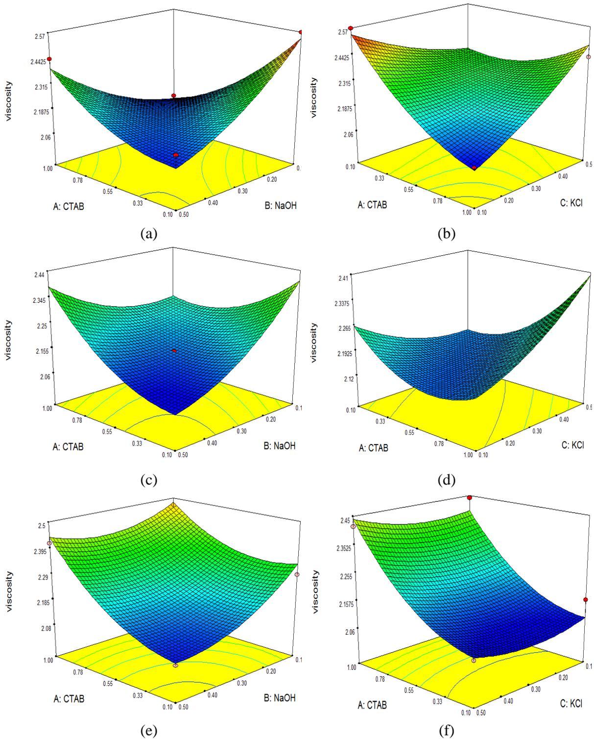
**Fig. 2.** Response surface plot for Viscosity (cP) of CTAB and NaOH at (a) 0.10 wt% of KCl, (b) 0.20 wt% of KCl, (c) 0.30 wt% of KCl. Also, CTAB and KCl at (d) 0.10 wt% of NaOH, (e) 0.20 wt% of NaOH, (f) 0.30 wt% NaOH.
