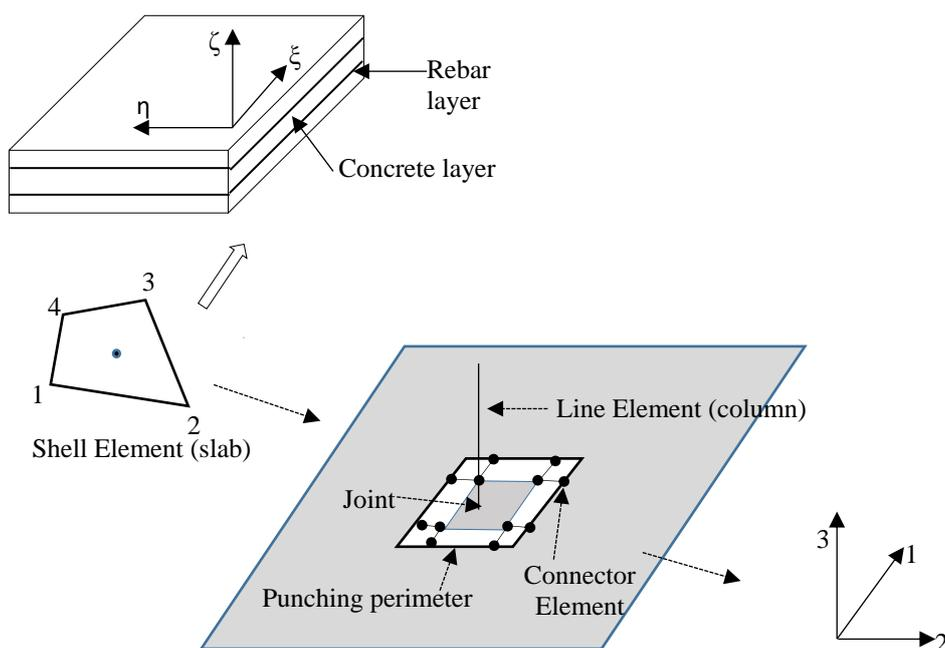
**Fig. 9.** Schematic sketch macro model for flat plate
