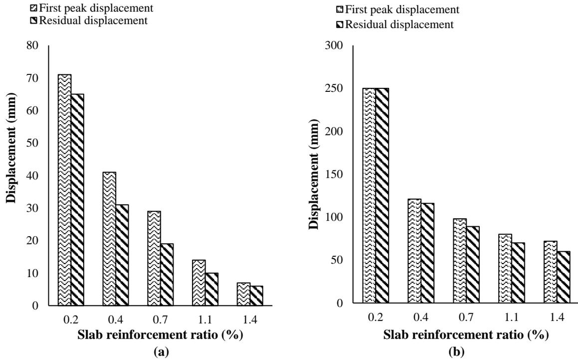
Fig. 6. Effect of reinforcement ratio: a) Flat slab structure and; b) Flat plate structure
