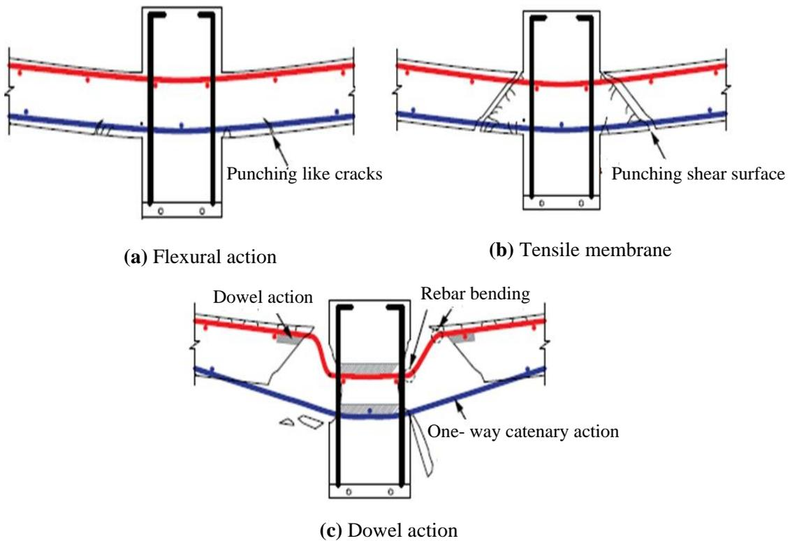
**Fig. 5.** Failure modes (Xue et al., 2018)
