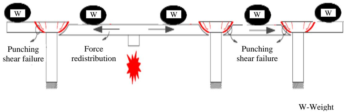
Fig. 1. Propagation of punching shear failure (Mitchell et al., 1984)
