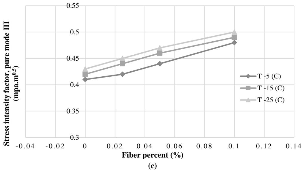
Fig. 7. Effect of test temperature on fracture toughness of asphalt mixture, loading rate of: a) 0.5 mm/min; b) 1 mm/min and; c) 5 mm/min
