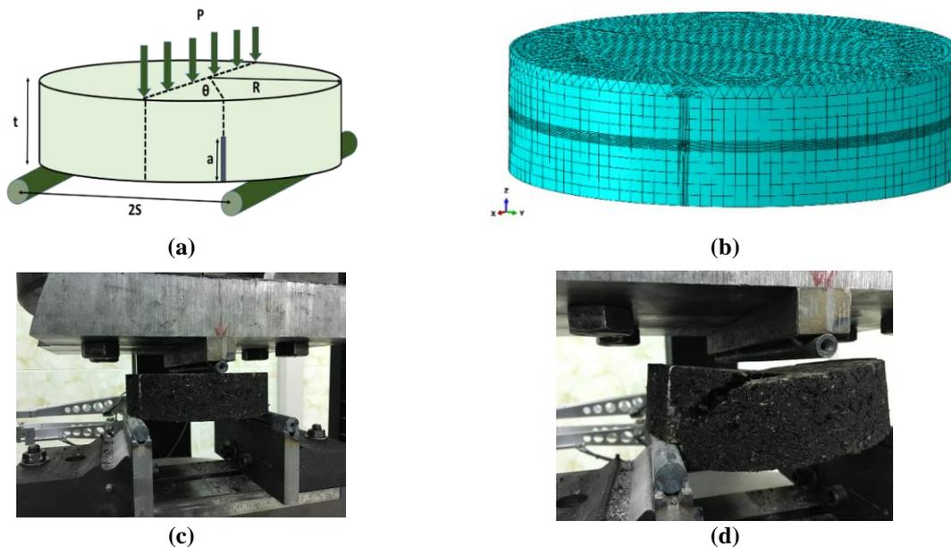
**Fig. 2.** a) Geometry specification and loading setup in the ENDB samples; Finite Element model in the ABAQUS code; Specification of loading setup; c) Before loading and; d) after loading
