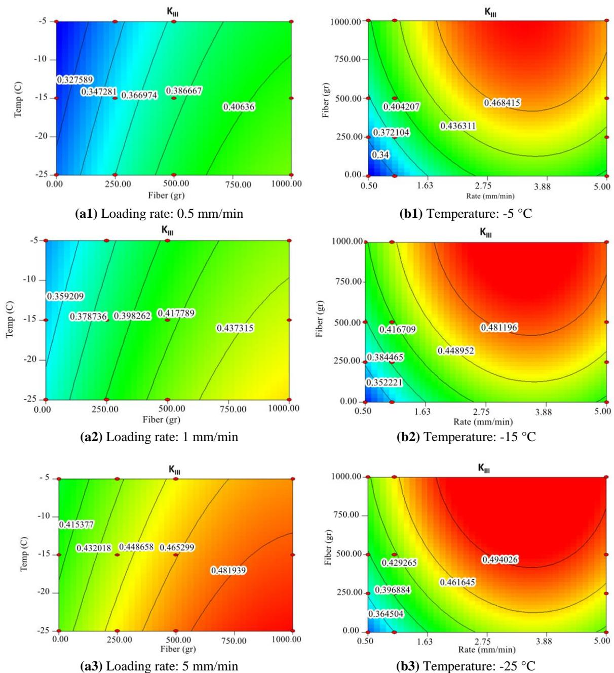
Fig. 10. The variations of prediction model obtained for the tested mode III ENDB specimens for: a) Different loading rates and; b) different temperatures
