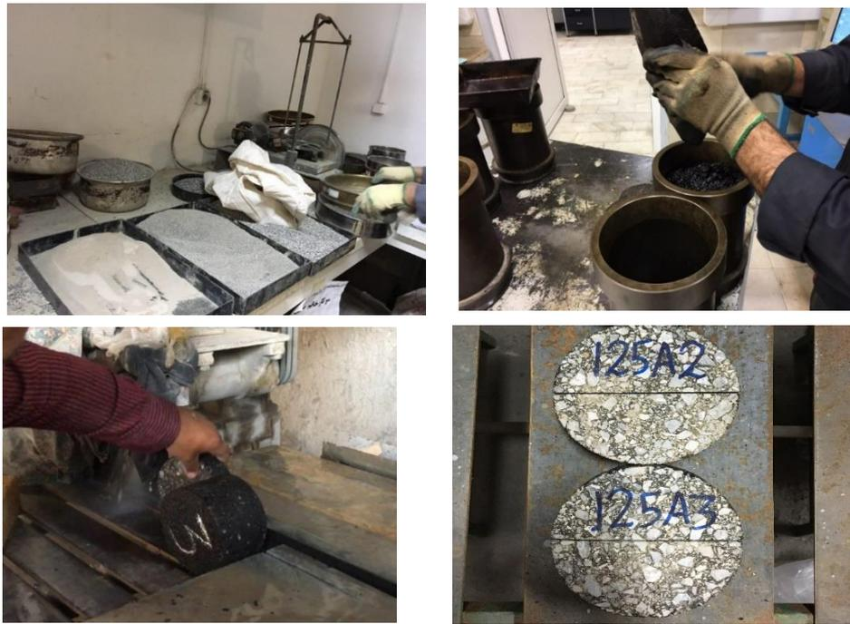
Fig. 3. Preparing and cutting process of ENDB specimen
