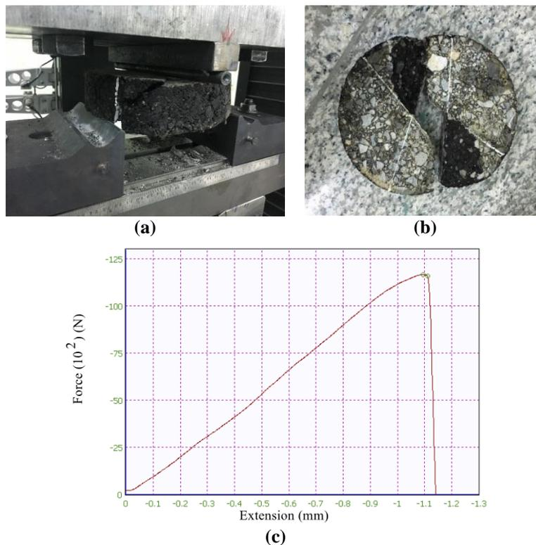
Fig. 4. An overview of performing the fracture test in pure mode III: a) loading setup; b) fracture section and; c) load-displacement curves
