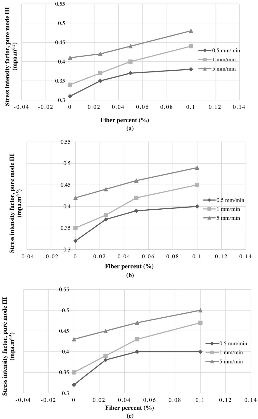
**Fig. 6.** Effect of the loading rate on mode III fracture toughness of asphalt mixture in different test temperatures: a) -5 °C; b) -15 °C and; c) -25 °C
