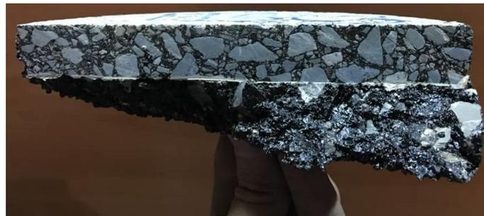
Fig. 8. The fracture propagation trajectory of tested asphalt mixture for the mode III fracture
