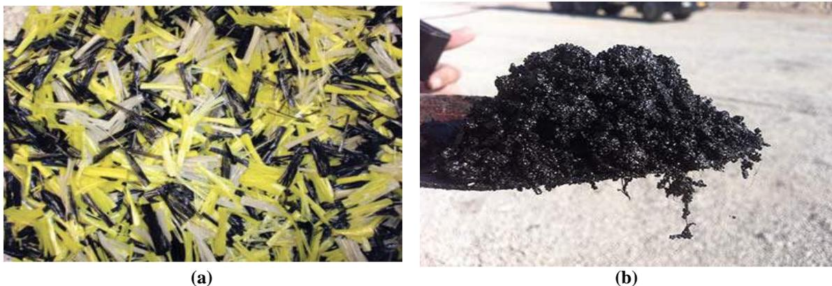
Fig. 1. Picture of: a) polyolefin – aramid fibers and; b) fiber reinforced asphalt mixture
