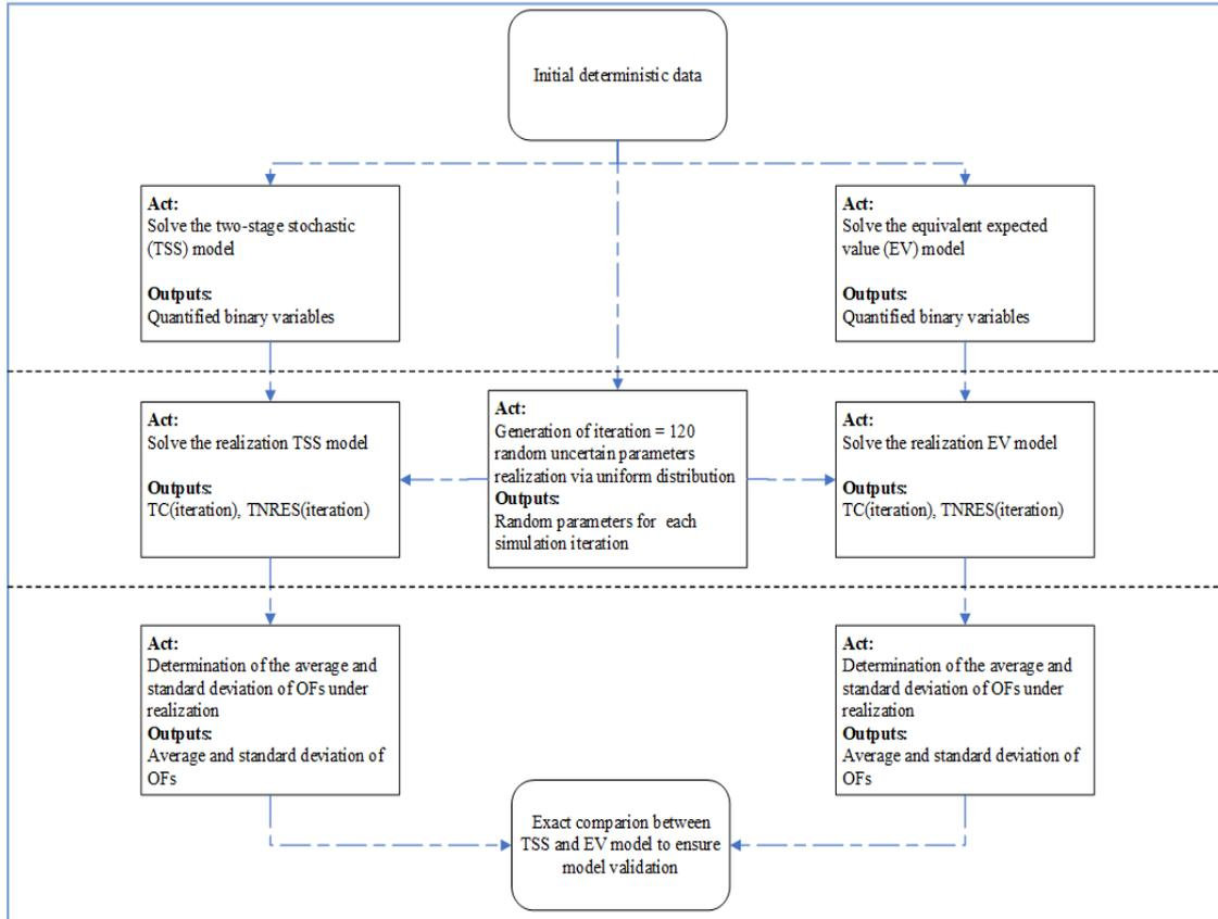
**Fig. 5.** The Implemented Simulation-Based Model Validation Approach
