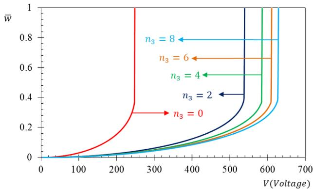
Figure 10. Effect of  $n_3$ , pull-in instability voltage ( $E_c = 70Gpa$ ,  $E_m = 70Gpa$ ,  $\alpha_m = 11 \times 10^{-6} 1/^\circ C$ ,  $\alpha_c = 23.1 \times 10^{-6} 1/^\circ C$ ,  $\nu = 0.3$ ,  $b = 1\mu m$ ,  $L = 100\mu m$ ,  $h = 1\mu m$ ,  $T = 5^\circ C$ ,  $\bar{l} = 0.01$ ,  $d = 1\mu m$ ,  $n_1 = 0$ ,  $n_2 = 0$ ,  $n_4 = 0$ )
