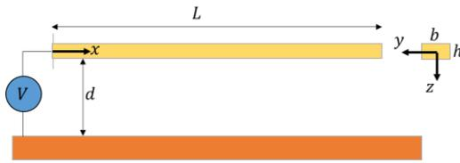
Fig. 1 Schematic of an electrostatic actuated FGM micro beam
