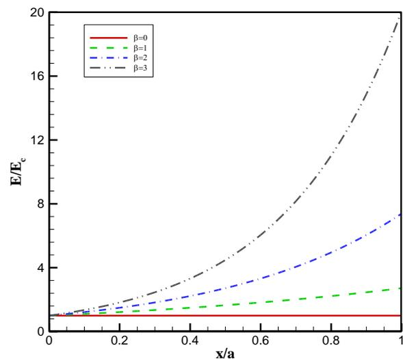
Figure 4. Distribution of module of elasticity versus  $x/L$  at  $z=-h/2$
