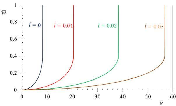
Figure 6. Effect of size parameter on pull-in instability voltage (  $E_c = 70Gpa \cdot E_m = 70Gpa \cdot \alpha_m = 11 \times 10^{-6} 1/^\circ C$
