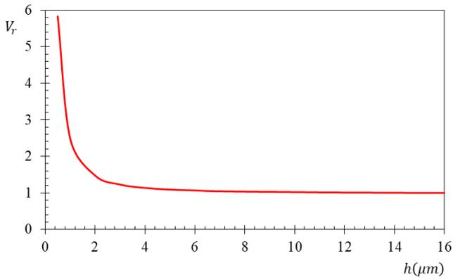
Figure 7. Effect of thickness on pull-in instability voltage (  $E_c = 70Gpa \cdot E_m = 70Gpa \cdot \alpha_m = 11 \times 10^{-6} 1/^\circ C$
