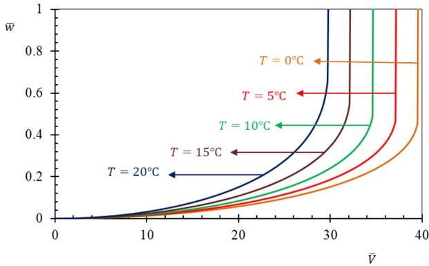
Figure 5. Effect of temperature on pull-in instability voltage (  $E_c = 70Gpa \cdot E_m = 70Gpa \cdot \alpha_m = 11 \times 10^{-6} 1/^\circ C$
