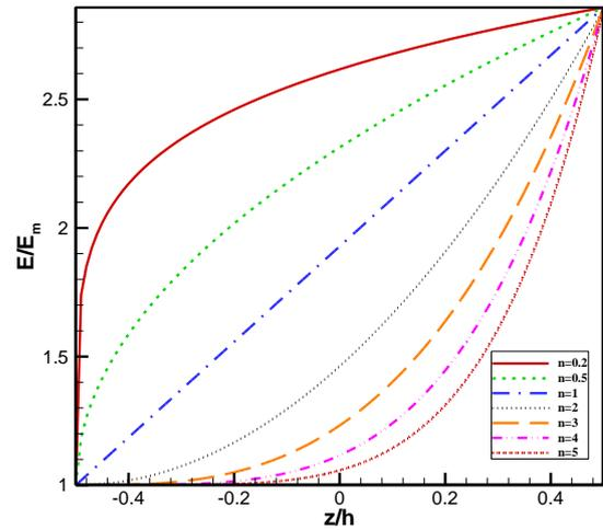
Figure 3. Distribution of module of elasticity versus  $z/h$  at  $x=0$
