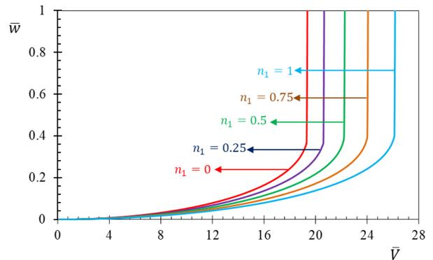
Figure 8. Effect of  $n_1$  pull-in instability voltage (  $E_c = 70Gpa \cdot E_m = 70Gpa \cdot \alpha_m = 11 \times 10^{-6} 1/^\circ C$
