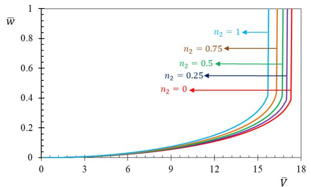
Figure 9. Effect of  $n_2$  pull-in instability voltage (  $E_c = 70Gpa \cdot E_m = 70Gpa \cdot \alpha_m = 11 \times 10^{-6} 1/^\circ C$
