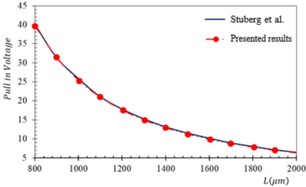
Figure 2. Comparison of Presented results obtained for pull-in voltage with those presented in the literatures ( $E = 169Gpa$ ,  $\nu = 0.3$ ,  $b = 50\mu m$ ,  $l = 0$ ,  $d = 1\mu m$  and  $h = 14.4\mu m$ )
