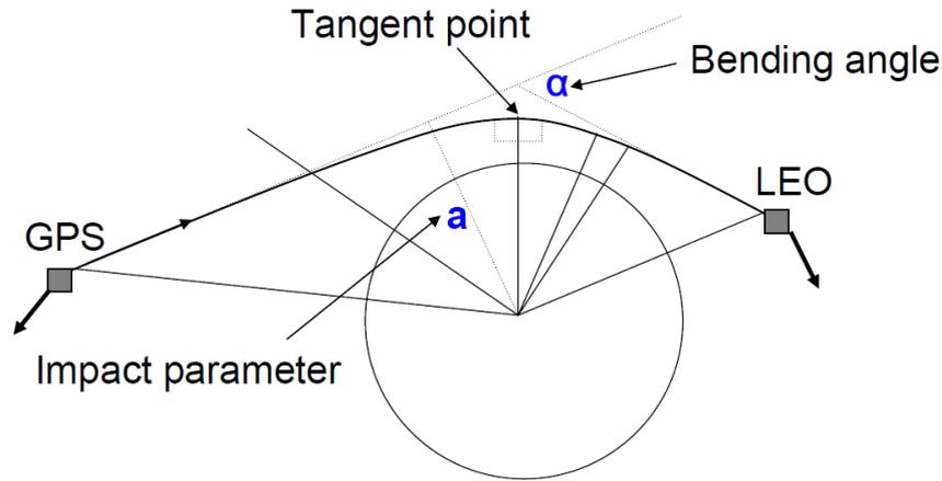
Figure 2. The geometry of a GPS RO measurement (Eyre, 2008).
