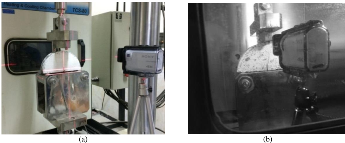
Fig. 4. SCB specimen and the testing setup: a) Using laser leveler; b) Temperature controlled chamber
