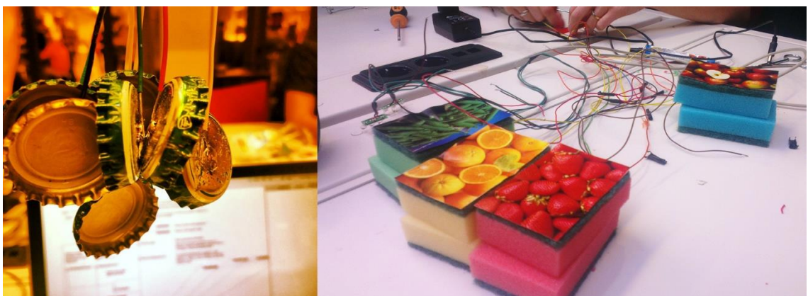
Figure 6: A simplified pressure sensor, made with beer bottle caps and sponges
