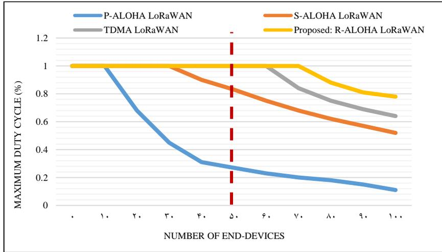
**Figure 6.** Maximum duty cycle vs. number of end-devices
