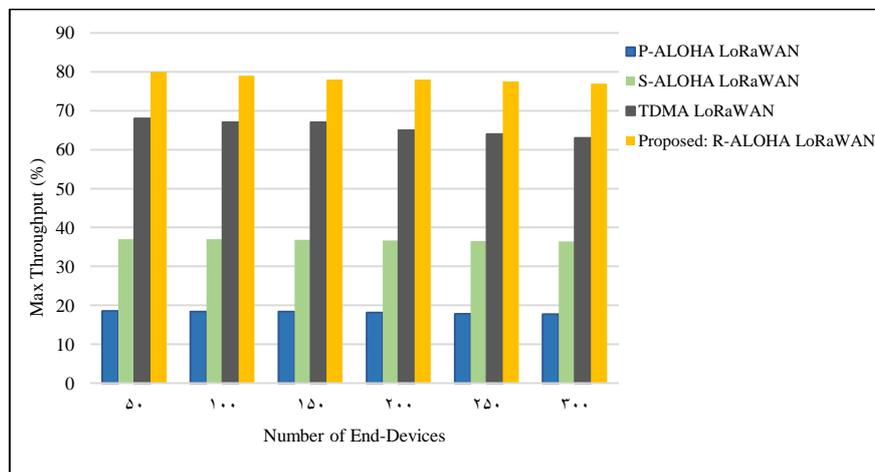
**Figure 5.** Maximum throughput vs. number of end-devices
