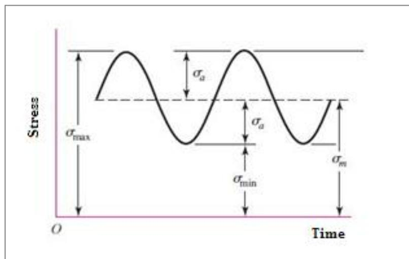
Figure 4: Stress-Time relation, fluctuating stress[8]
