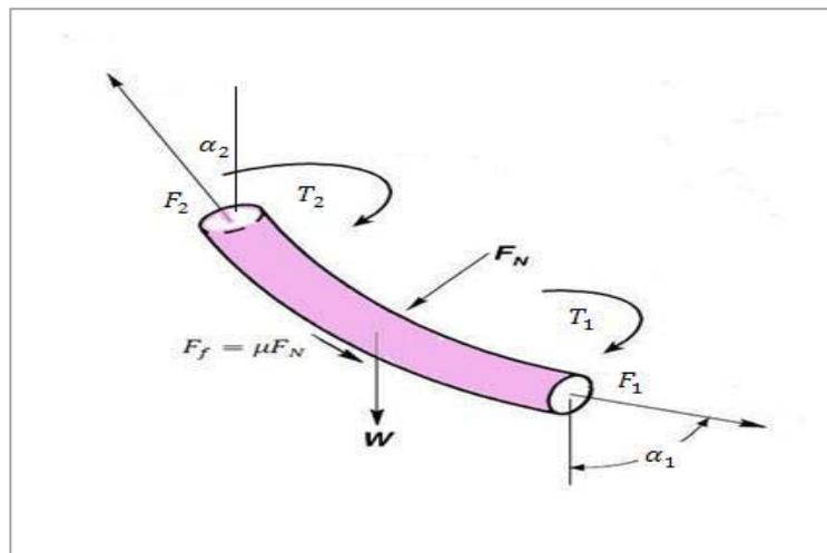
Figure 2: Drill string in curved section
