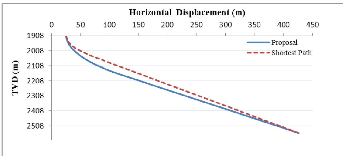
Figure 8: Comparison between proposed & shortest well path
