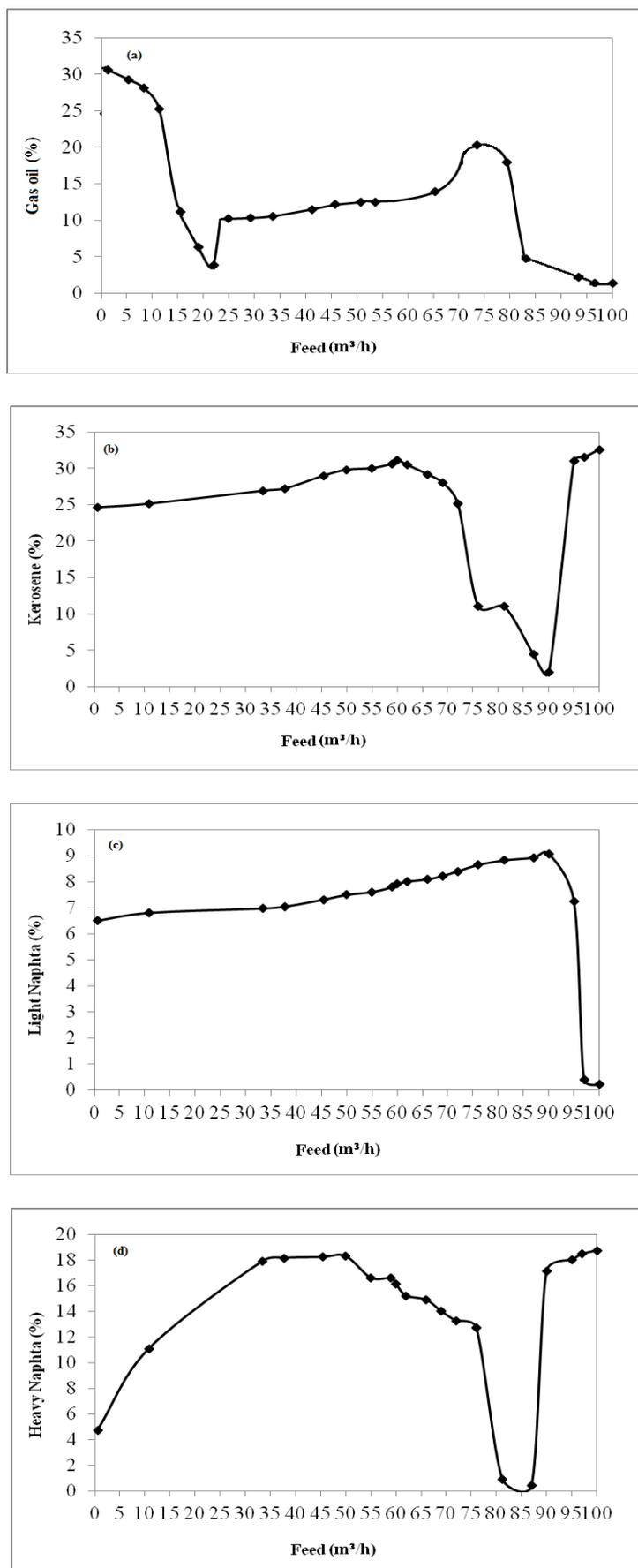
Figure 8: The effect of total feed flow rate on the volume percent of (a) gas oil, (b) kerosene, (c) LN, and (d) HN
