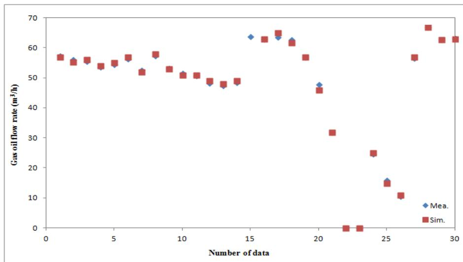
Figure 3: Comparison of measured flow rate of gas oil with values predicted by trained ANFIS
