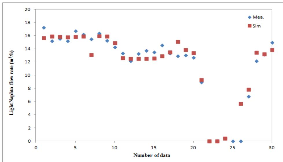
Figure 5: Comparison of measured flow rate of LN with values predicted by trained ANFIS
