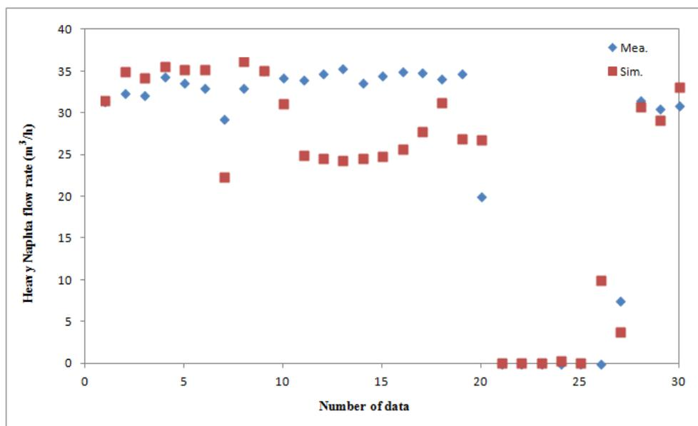
Figure 6: Comparison of measured flow rate of HN with values predicted by trained ANFIS
