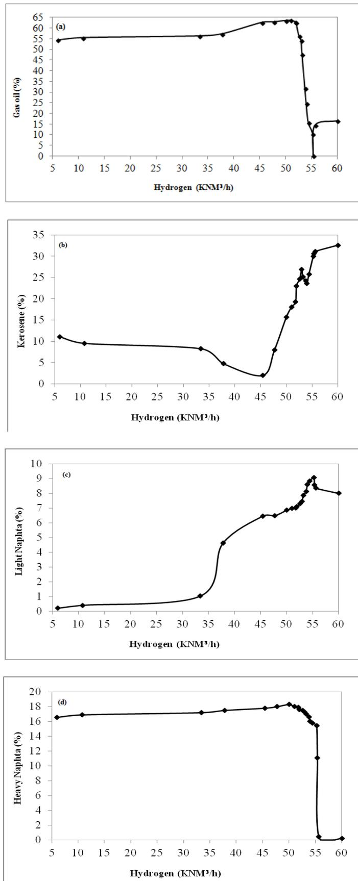
**Figure 9: The effect of hydrogen flow rate on the volume percent of (a) gas oil, (b) kerosene, (c) LN, and (d) HN**
