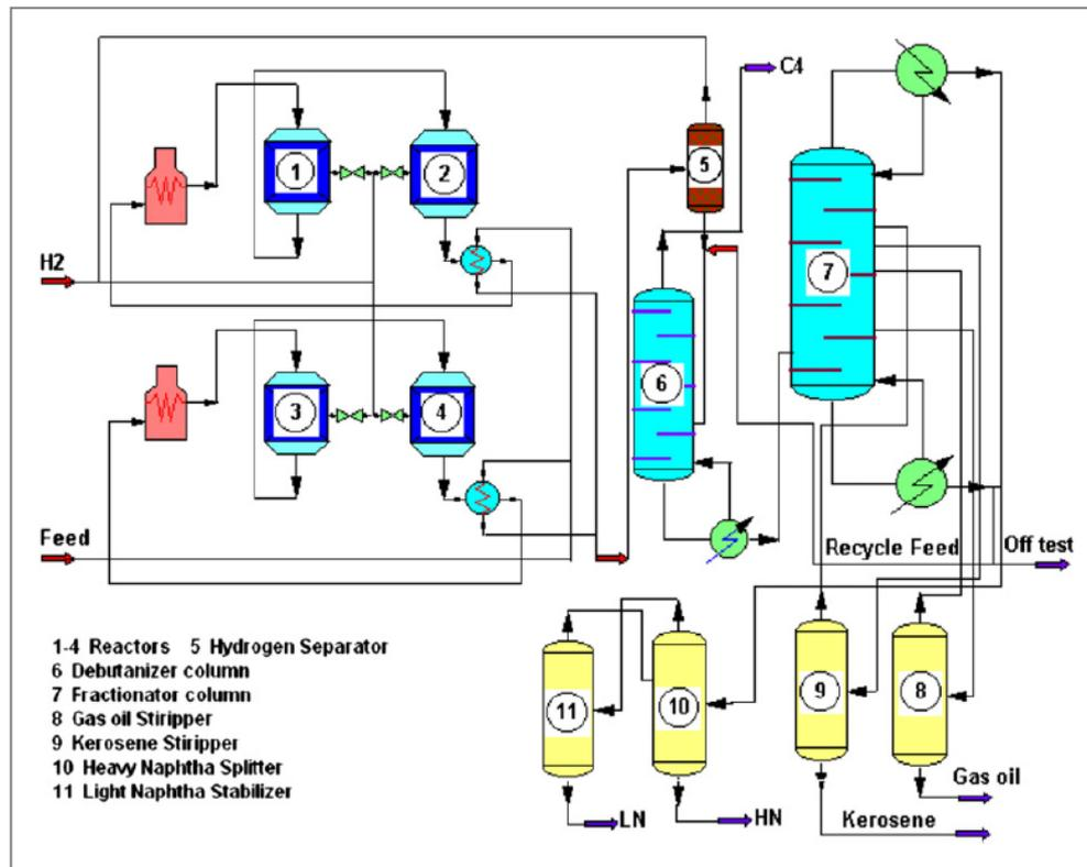
Figure 1: Process flow diagram of a hydrocracking unit (Isomax unit)
