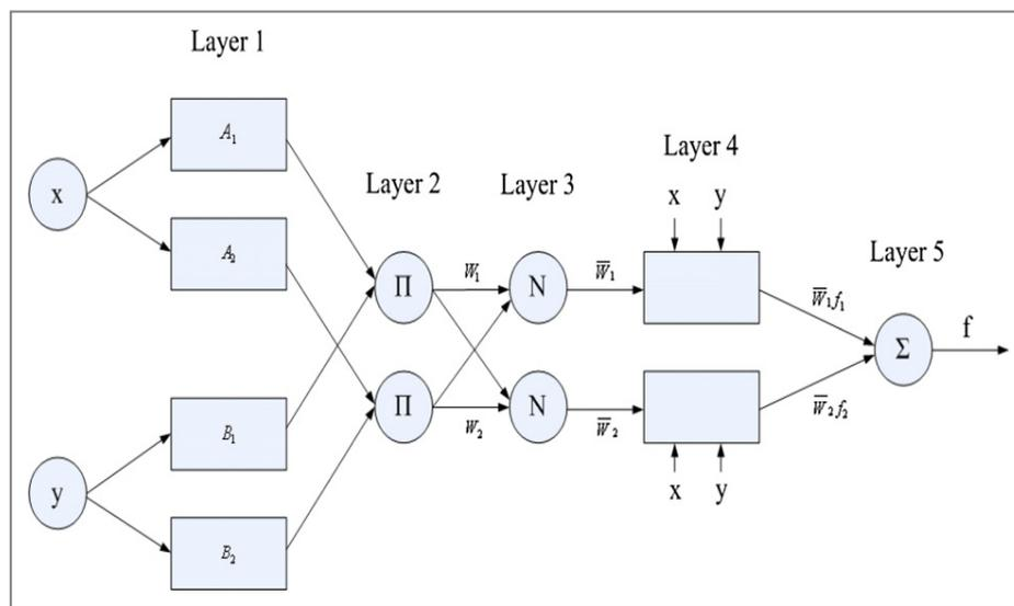
**Figure 2: Adaptive Neuro-Fuzzy Inference System (ANFIS) structure**
