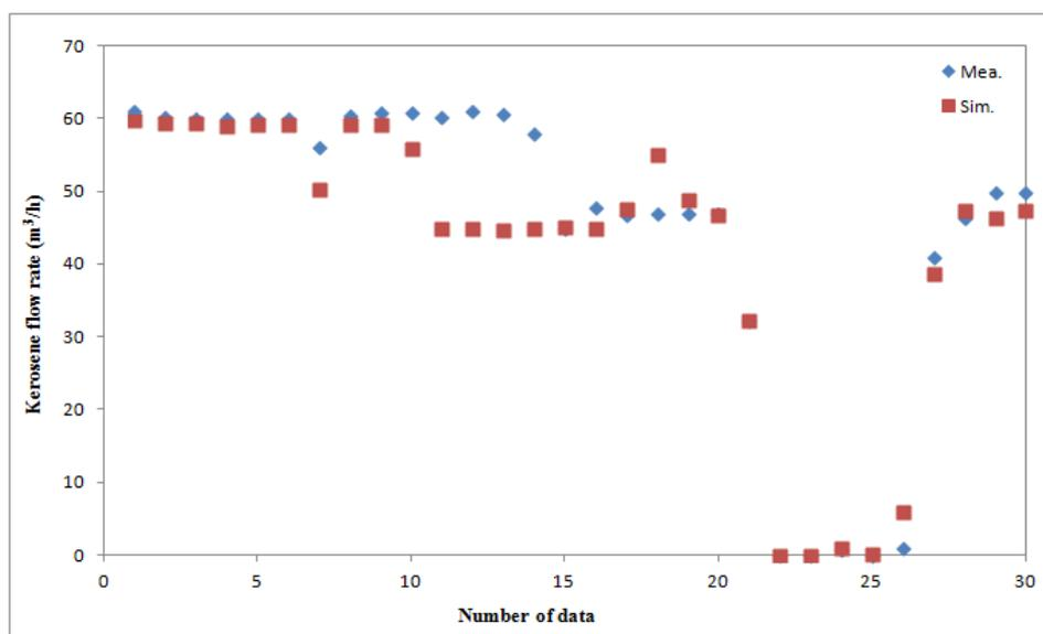
Figure 4: Comparison of measured flow rate of kerosene with values predicted by trained ANFIS
