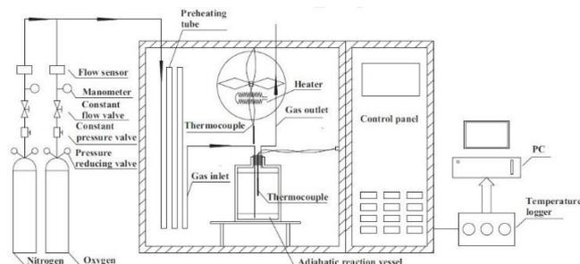
Fig. 5. A schematic diagram of the apparatus applied for the oxidation test system.
