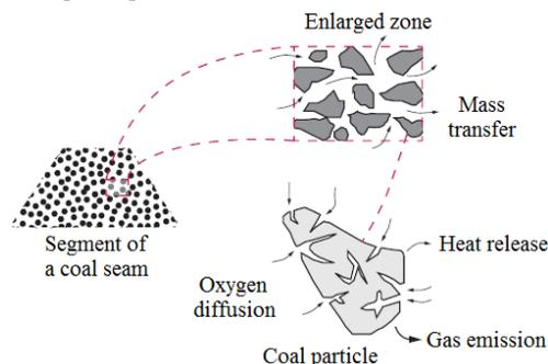
Fig. 1. Schematic illustration of the coal oxidation process.
