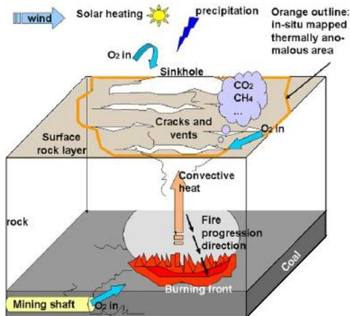
Fig. 2. Different aspects of pollution due to spontaneous coal combustion [36].
