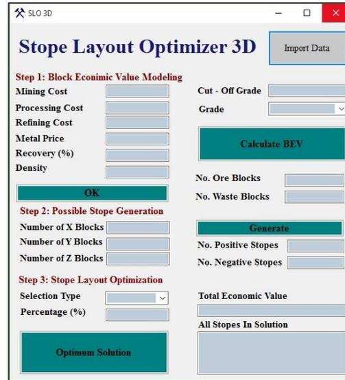
**Fig 5.** Stope Layout Optimizer 3D.
