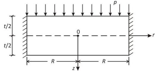
Figure 1: Thick circular plate of radius  $R$  subject to uniformly distributed transverse load,  $p$  on the top surface
