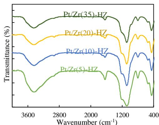
**Figure 2.** FTIR spectra for the powder Pt/Zr(x)-HZ catalysts
