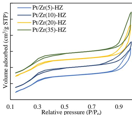
**Figure 4.** BET isotherms of platinumated Zr(x)-HZ catalysts
