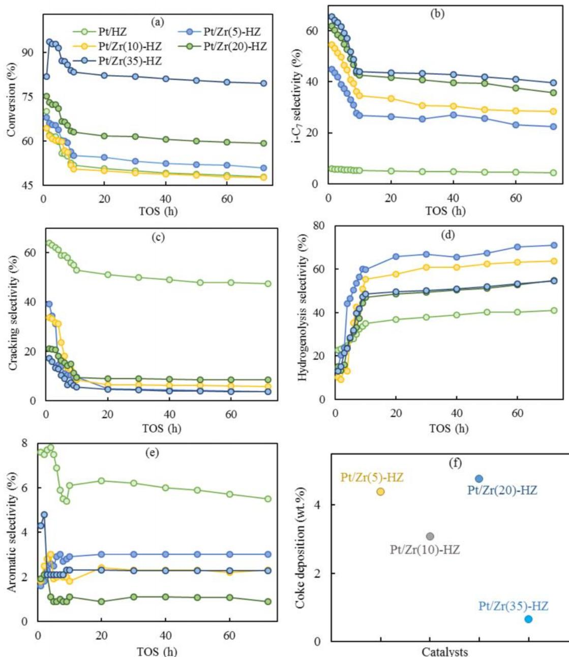
**Figure 6.** The stability of Pt/Zr(x)-HZ catalysts during 72 h on stream (TOS) at 400 °C for various reactions of reforming: (a) conversion and selectivity to (b) i-C<sub>7</sub> isomers, (c) cracking, (d) hydrogenolysis, (e) aromatic and (f) coke deposition.
