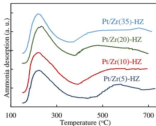
**Figure 5.** NH<sub>3</sub>-TPD diagrams for platinumated Zr(x)-HZ catalysts
