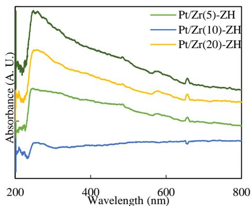
**Figure 3.** UV-vis DRS of the Pt/Zr(x)-HZ catalysts
