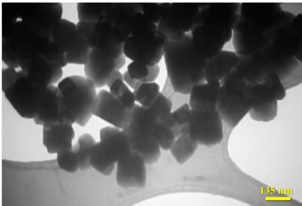
**Figure 3.** TEM image of the as-synthesized Fe-doped CeO<sub>2</sub> NPs
