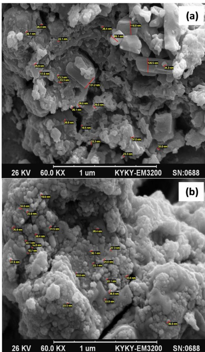
**Figure 2.** FESEM images of the (a) as-prepared (b) annealed Fe-doped CeO<sub>2</sub> NPs at 500 °C
