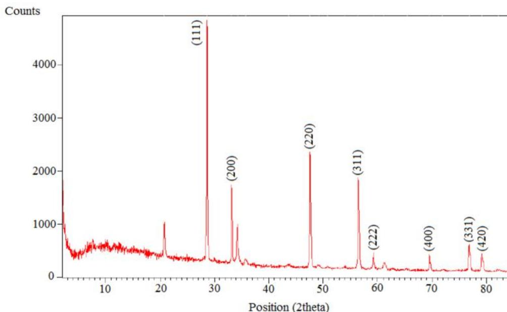
Figure 1. XRD pattern of annealed Fe-doped  $\text{CeO}_2$  sample
