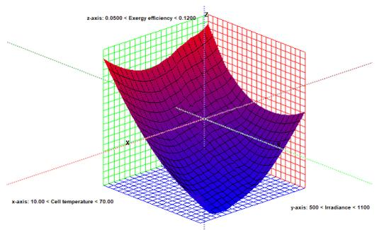
Figure 14. Variation of exergy efficiency with cell temperature and irradiance
