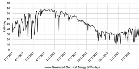
Figure 3. Simulated daily electrical energy generation of BIPV system by PVsyst software
