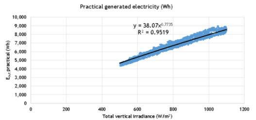
Figure 8. Data mining for practical energy generation vs. vertical solar irradiance
