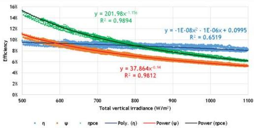
Figure 10. Variation of power conversion, energy and exergy efficiencies with vertical solar irradiance
