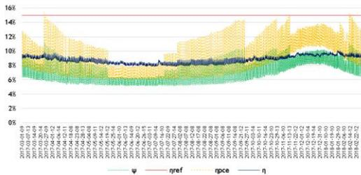
Figure 5. Reference, power conversion, energy and exergy efficiencies of BIPV modules in quasi-dynamic conditions
