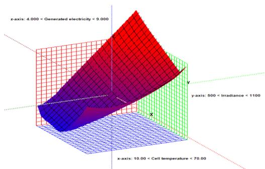
Figure 11. Variation of practical energy generation with cell temperature and irradiance
