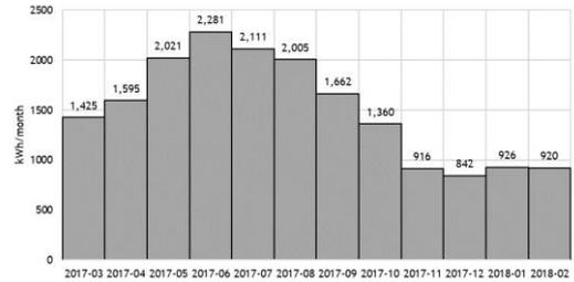
Figure 2. Simulated monthly electrical energy generation of BIPV system by PVsyst software
