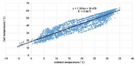
Figure 6. Data mining of PV cell temperature vs. ambient temperature
