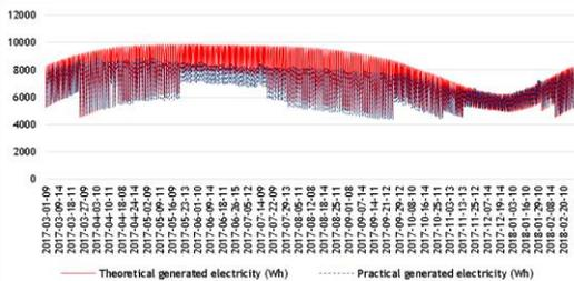
Figure 4. Calculated theoretical and practical energy generation of BIPV modules in quasi-dynamic conditions
