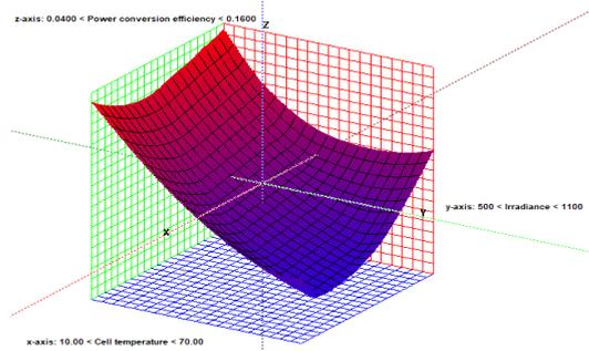
Figure 12. Variation of power conversion efficiency with cell temperature and irradiance
