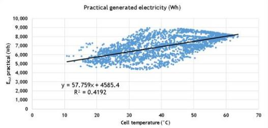
Figure 7. Data mining for practical energy generation vs. cell temperature
