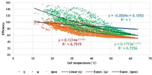
Figure 9. Variation of power conversion, energy and exergy efficiencies with cell temperature
