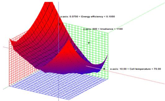
Figure 13. Variation of energy efficiency with cell temperature and irradiance
