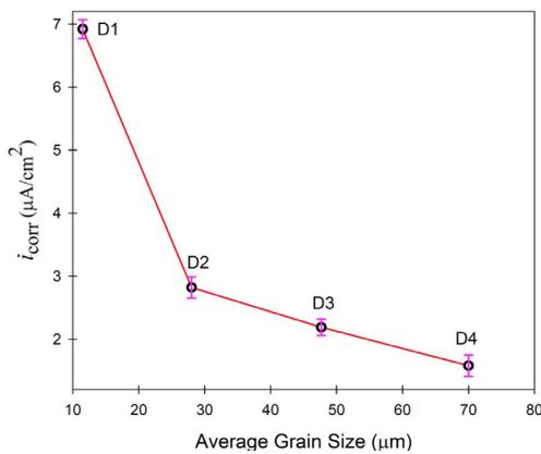
Fig. 4- Values of  $i_{corr}$  versus average grain size.
