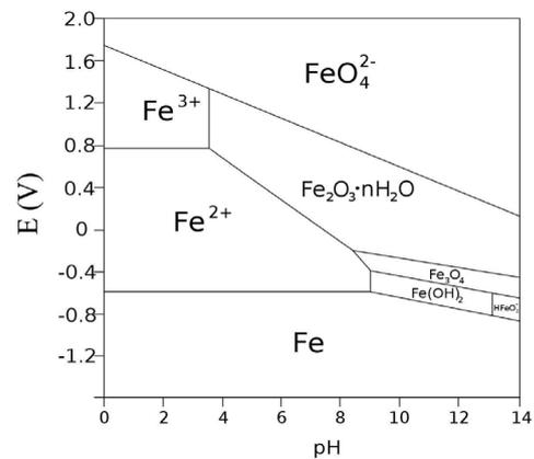
Fig. 5- Pourbaix diagram (simplified potential-pH) of iron [13].
