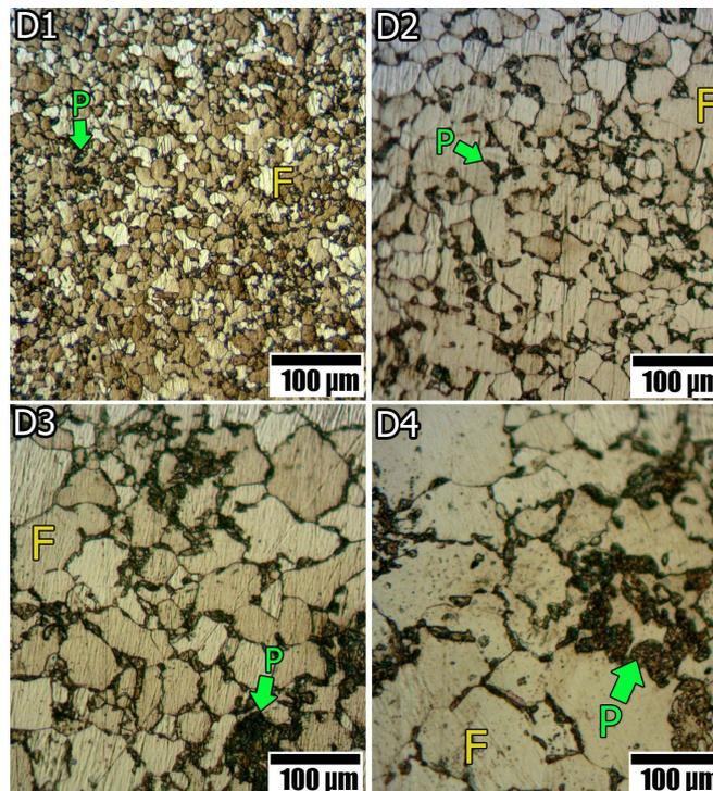
Fig. 1- Micrographs of the processed samples, where F and P denote the ferrite grains and pearlite colonies, respectively.
