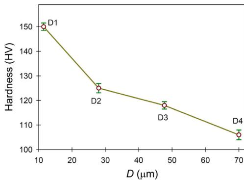
Fig. 2- Hardness versus average grain size.
