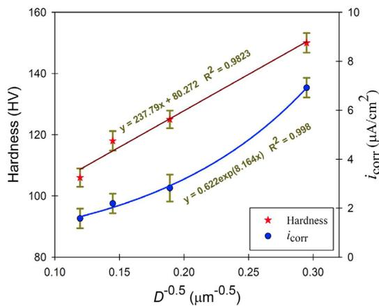
Fig. 6- Dependency of hardness and  $i_{\text{corr}}$  on average grain size.
