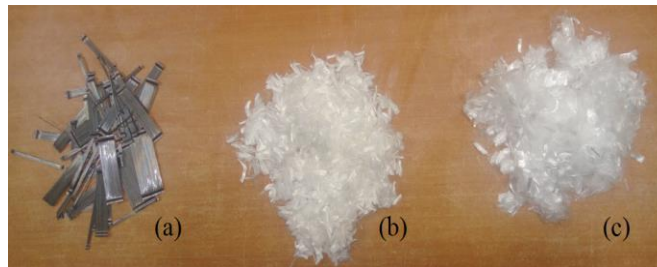
Fig. 2. Fibers used in this study: a) macro fiber steel, b) micro fiber polypropylene, and c) micro fiber glass
