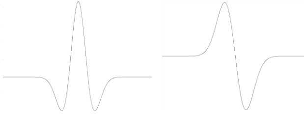
Figure 6. Two mother wavelets used as the activation functions for the WNN. Mexican Hat (left) and Gaussian Gradient (right).
