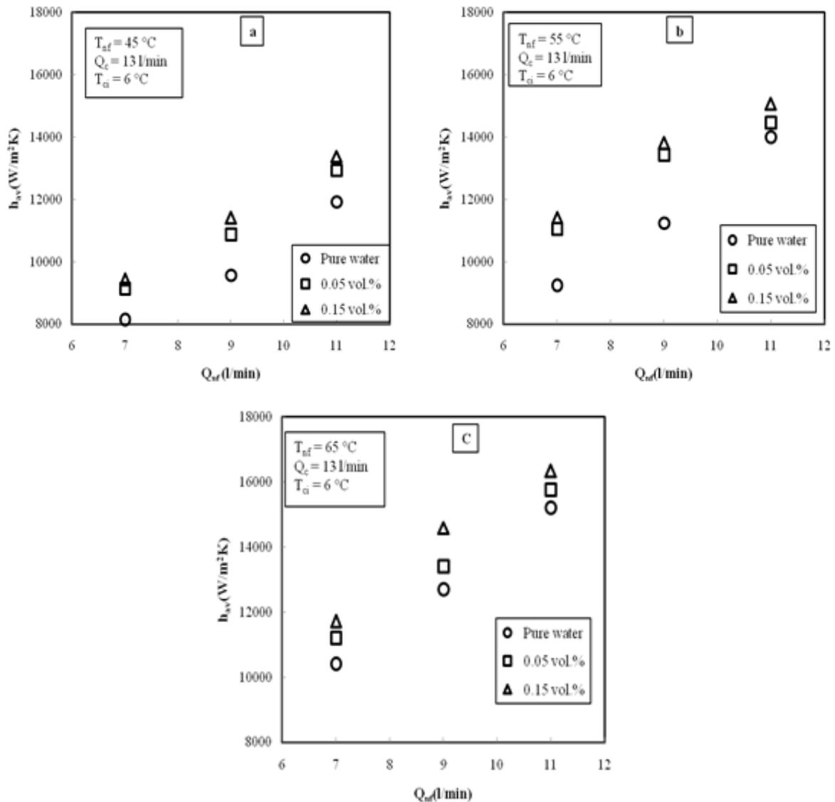
**Fig. 4.** The average heat transfer coefficient of  $\gamma$ - $\text{Al}_2\text{O}_3$ /water nanofluid as a function of the nanofluid flow rate at different nanofluid concentrations and inlet temperatures of a) 45 °C, b) 55 °C, c) 65 °C
