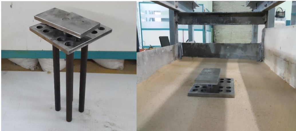
Fig. 3. Pile raft foundation (raft and pile with platform)
