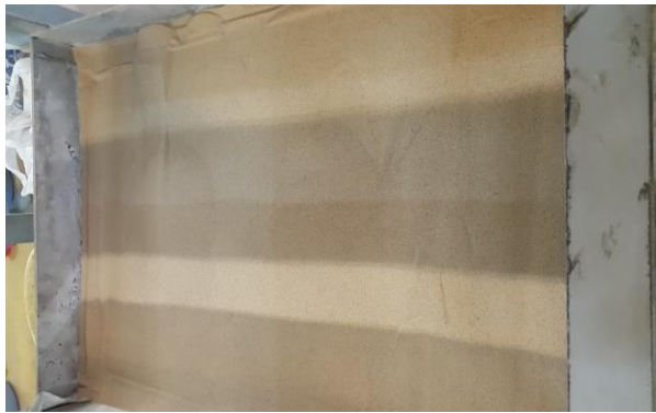
a) Step 1. Filing the box with sand (80 cm)
