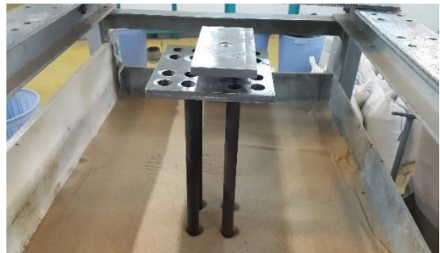
f) Step 3. Driving the piles in sandy layer
