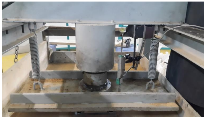
Fig. 2. Loading system (hydraulic jack with bearing plate)
