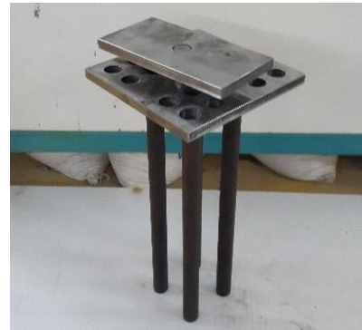
d) Step 2. Piled raft assembling
