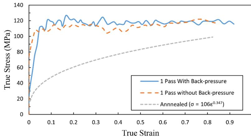
Fig. 13- True Stress Vs True Strain curve of the samples with and without back-pressure.
