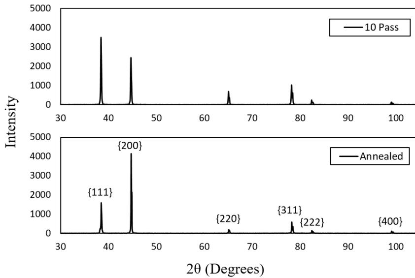
Fig. 14- XRD patterns of the 10<sup>th</sup> pass processed and annealed samples.
