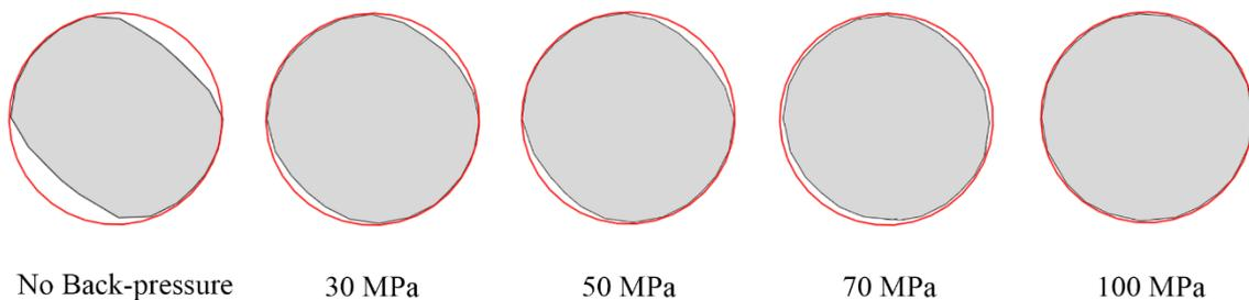
Fig. 5- Effect of different amounts of back-pressure at the sample's cross-section obtained by FEM.
