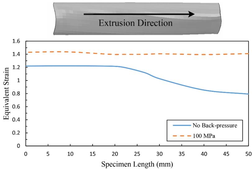
Fig. 8- The equivalent strain (PEEQ) distribution curve throughout the sample's length after the process.
