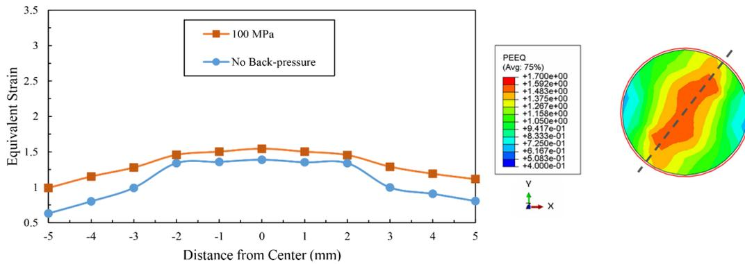
Fig. 6- the distribution of the equivalent strain (PEEQ) on the cross-section of the sample after CSSE.
