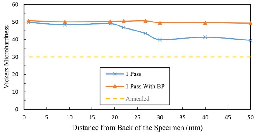
Fig. 11- Distribution of hardness in the length of the specimens with and without back-pressure.
