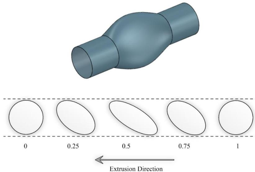
Fig. 1- (a) Schematic design of CSSE's deformation channel and (b) the geometry of the material's cross-section during deformation.
