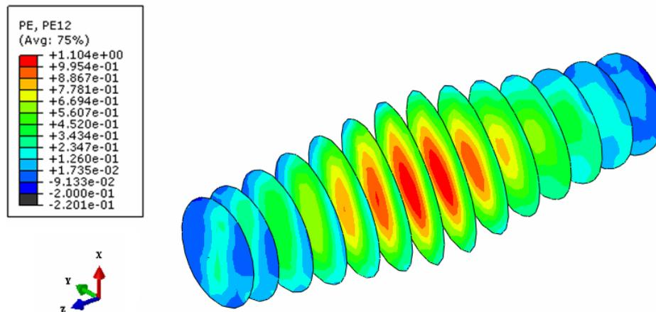
Fig. 2- Shear strain distribution in the sample's cross-section throughout the deformation channel.
