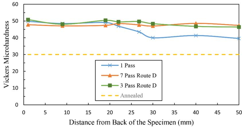
Fig. 12- Distribution of hardness in the length of the specimens at different passes.
