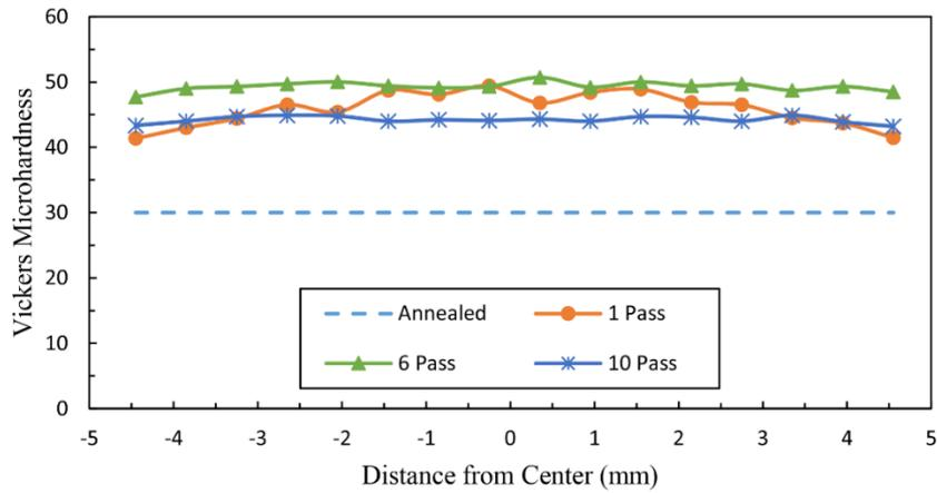
Fig. 10- Hardness distribution on the cross-section of samples with different passes of route D.
