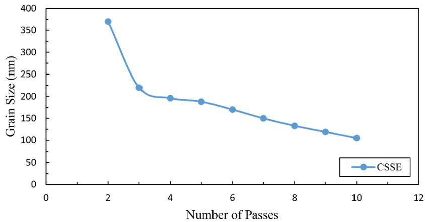
Fig. 15- Crystallite Size Vs Different Number of passes of the CSSE process.
