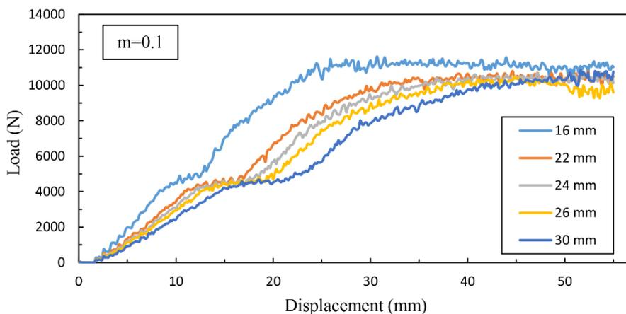
Fig. 3- The load-displacement curve obtained from simulations of the CSSE process with different deformation channel lengths.
