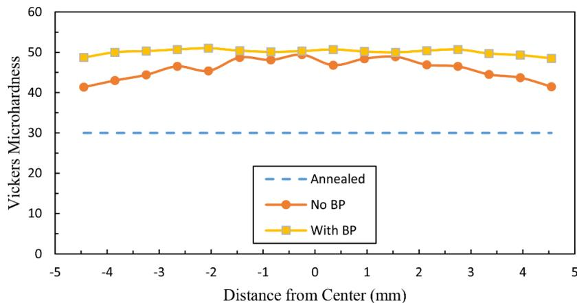
Fig. 9- Hardness distribution on the cross-section of the annealed sample and samples after one pass of CSSE with and without back-pressure.
