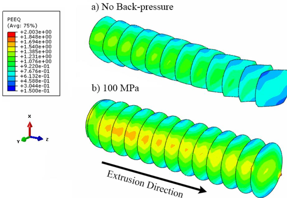
Fig. 7- Sectioned view of equivalent strain in processed samples with a) 0 MPa and b) 100 MPa of back-pressure.
