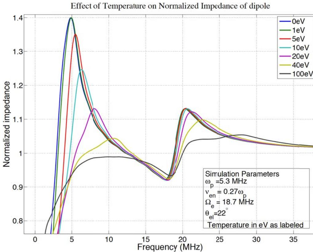
**Figure 3.** Impedance of a dipole antenna in a homogeneous plasma for different values of electron temperature as simulated by PF-FDTD.
