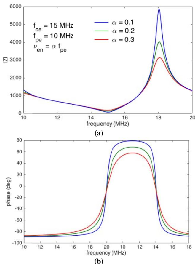
**Figure 1.** Variation effect of electron density (electron plasma frequency) on antenna input impedance a) amplitude and b) phase using Balmain theoretical model associated with varying electron neutral collision frequency.
