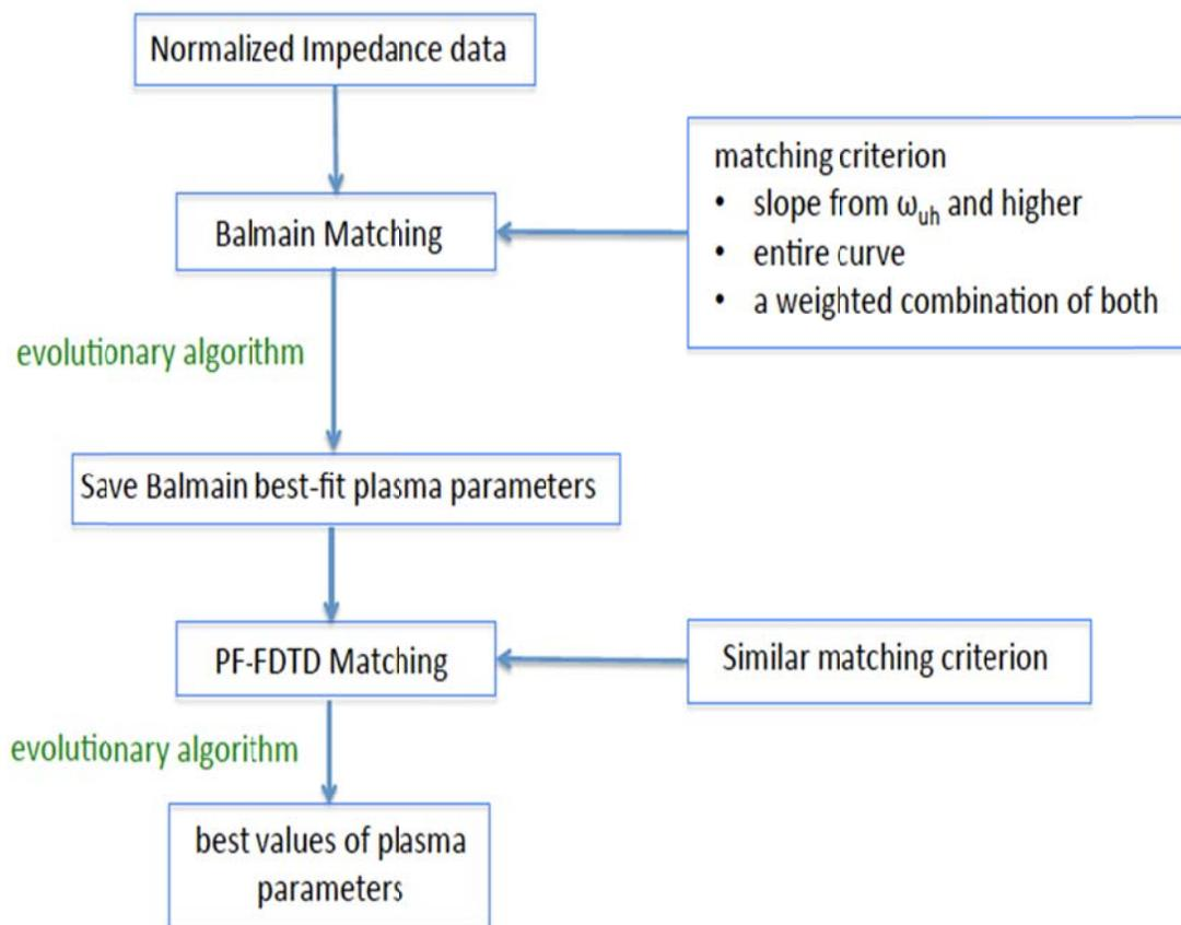
**Figure 4.** Data reduction technique using the measured impedance data and comparison with the Balmain theoretical model and PF-FDTD model.
