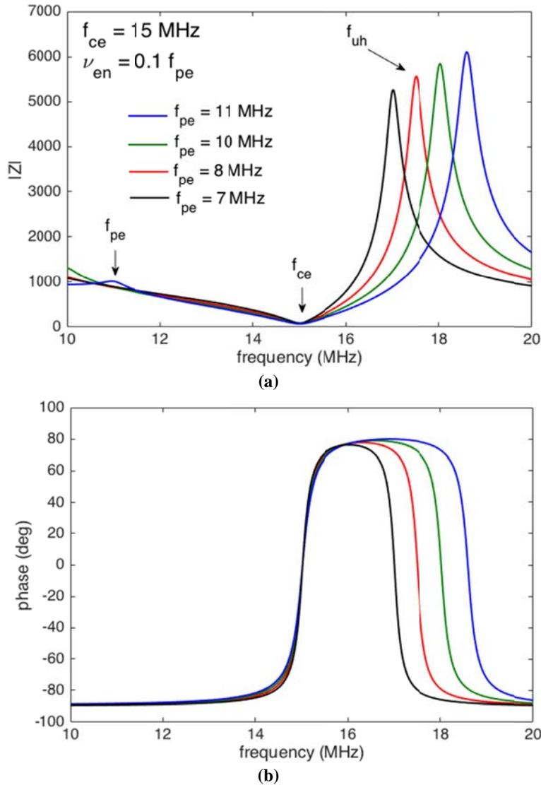
**Figure 2.** Variation effect of electron-neutral collision frequency on antenna input impedance a) amplitude and b) phase using Balmain theoretical model associated with varying electron plasma frequency.
