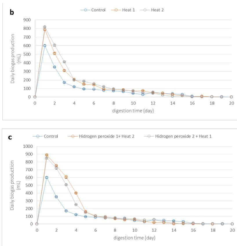
**Fig. 3.** Daily biogas production in a) pre-treated reactors with hydrogen peroxide, b) pre-treated reactors with heat, and c) pre-treated reactors with combined hydrogen peroxide and heat. Error bars represent standard errors, obtained from triplicate tests.
