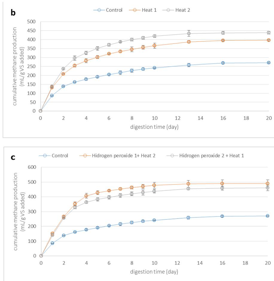
**Fig. 4. Cumulative methane generation in a) pre-treated reactors with hydrogen peroxide, b) pre-treated reactors with heat, and c) pre-treated reactors with combined hydrogen peroxide and heat. Error bars represent standard errors, obtained from triplicate tests.**
