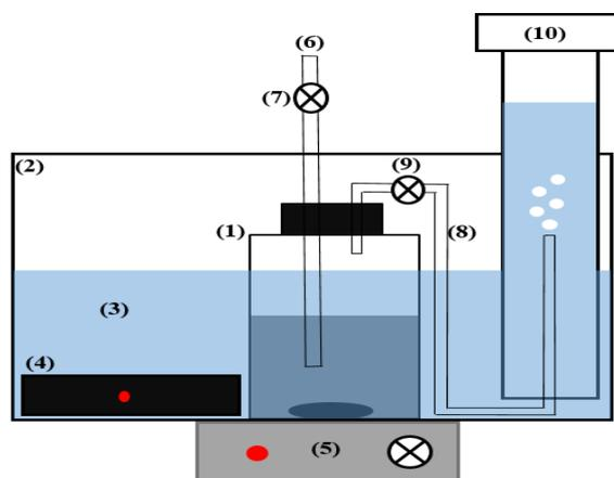
**Fig. 1. Schematic depiction of the experimental system: 1) biochemical methane potential reactor, 2) aquarium, 3) saturated and acidified water, 4) automatic heater, 5) magnetic stirrer, 6) sampling pipe, 7) sampling control valve, 8) biogas collecting pipe, 9) biogas control valve, and 10) graduated cylinder**
