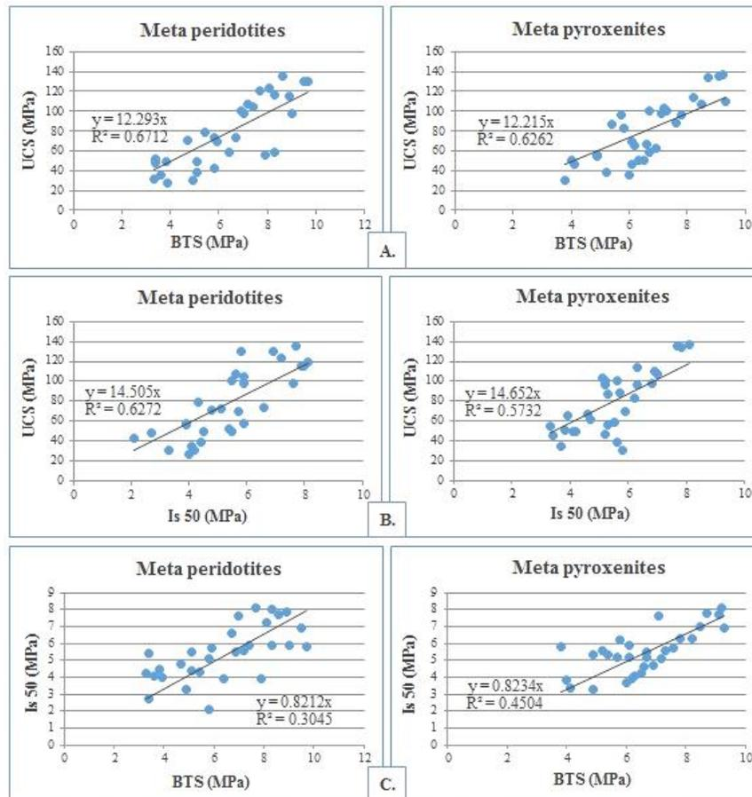
Figure 6. The relationship between A. UCS and BTS, B. UCS and  $Is_{50}$ , and C. BTS and  $Is_{50}$
