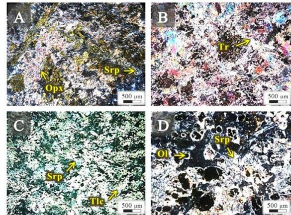
Figure 3. A. Increased fracture and microfracture in orthopyroxene (Opx) with increased serpentinization; B. Conversion of Clinopyroxene to Tremolite (Tr); C. Conversion of Orthopyroxene to Talc (Tlc); and D. Maintaining Olivine circular molds by increasing serpentinization
