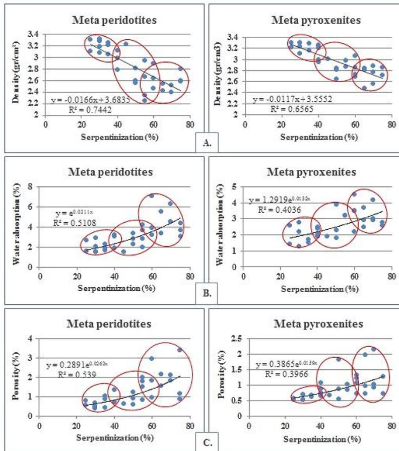
Figure 8. Variations of A. density ( $gr/cm^3$ ), B: water absorption (%), and C: porosity (%) relative to the serpentinization percentage
