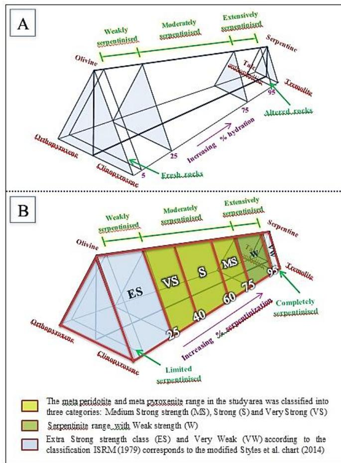
Figure 5. A. Different degrees of serpentinization in ultramafic rocks (Styles *et al.*, 2014); B. Modified Styles *et al.* chart (2014) and the relationship between the percentage of serpentinization and UCS based on the three classes of resistance MS, S, and VS in meta-period types and meta-pyroxenites
