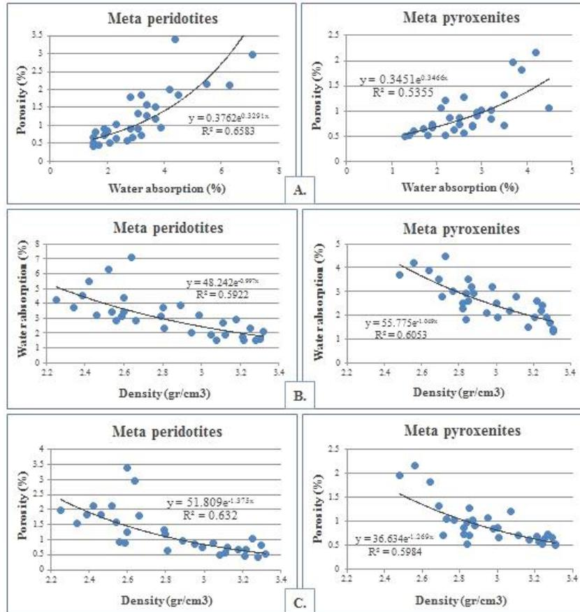
Figure 9. The relationship between: A. porosity (%) and water absorption (%), B: water absorption (%) and density (gr/cm<sup>3</sup>), C: porosity (%) and density (gr/cm<sup>3</sup>)
