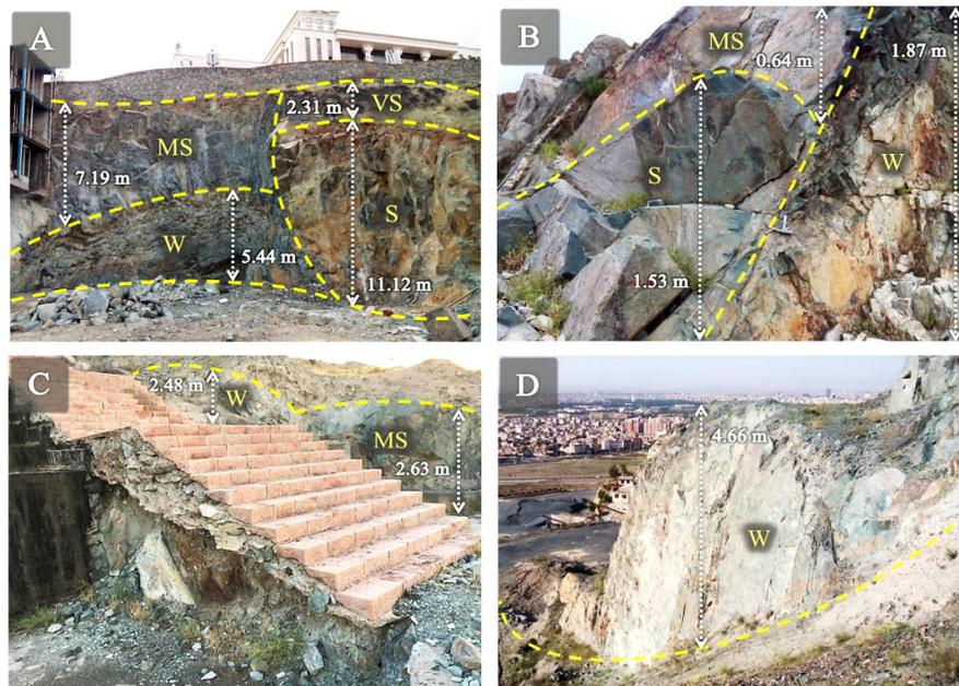
Figure 12. Examples of field behavior of rock mass in the studied area. A: resistance classes VS, S, MS, and W; B: resistance classes S, MS, and W; C: Resistance classes MS, W; and D: Resistance class W.
