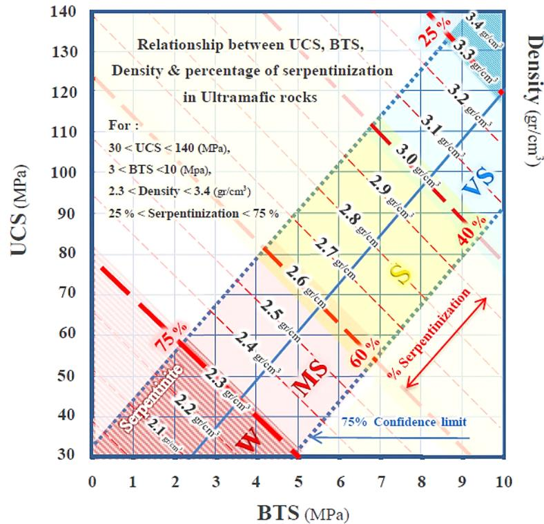
Figure 11. The relationship between UCS, BTS, and density with respect to the percentage of serpentinization in ultramafic rocks
