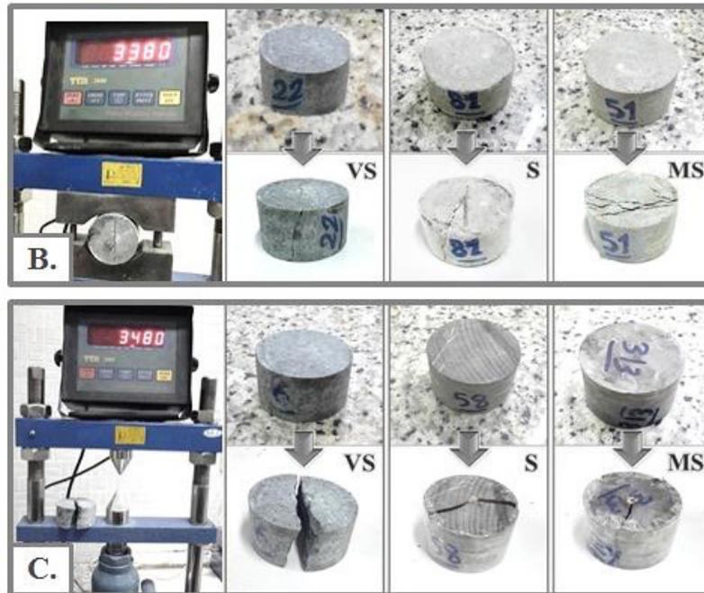
Figure 7. A: Examples of UCS in three resistance classes before and after the test, B: Examples of (BTS) in three resistance classes before and after the test, and C: Examples of ( $I_{s50}$ ) in three resistance classes before and after the test and their failure types
