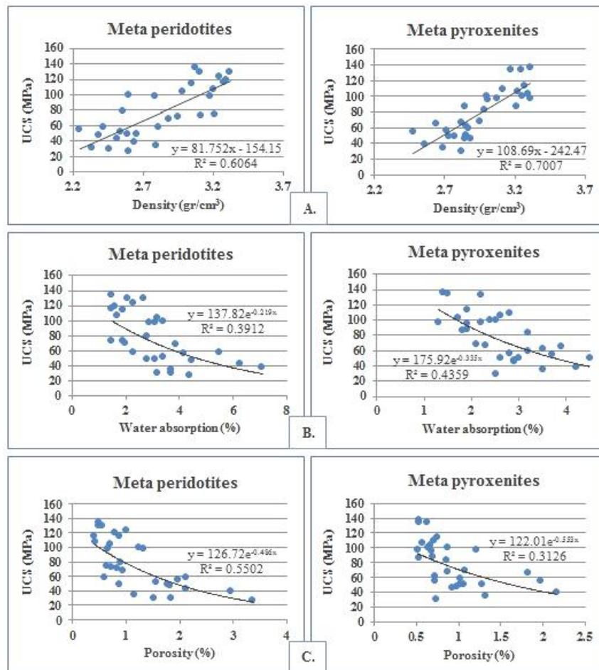
Figure 10. The relationship between A: UCS (MPa) and density (gr/cm<sup>3</sup>), B: UCS (MPa) and water absorption (%), C: UCS (MPa) and porosity (%)
