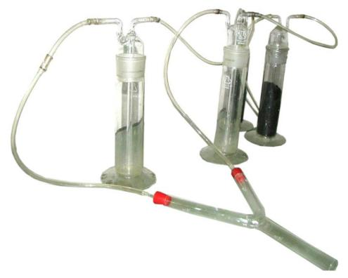
Figure 1. Y-tube olfactometer for recording responses of olive fruit fly females to volatiles.
