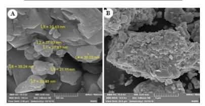
Figure 1. SEM of CuO-NPs. A. nm scale. B. µm scale
