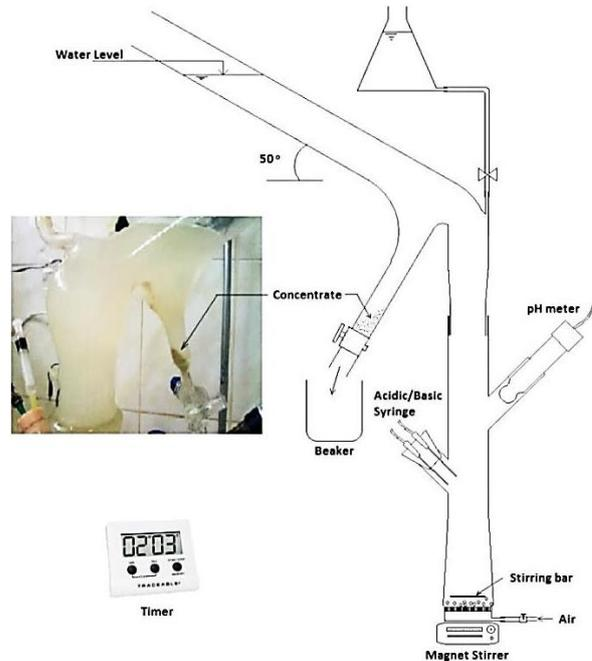
Fig. 3. Scaled up flotation cell as a modified large scale Hallimond tube [23].
