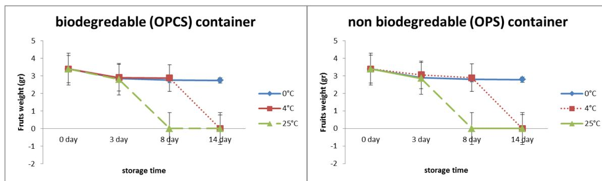
Fig. 2. Interaction of storage time and temperature on fruit weight of thornless blackberry in OPCS (left) and OPS (right) containers.
