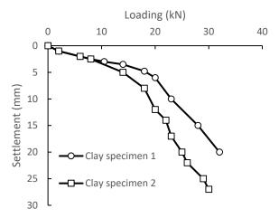
Fig. 14. Load-settlement behavior of clay specimens
