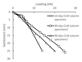
Fig. 15. Load-settlement behavior of CLM column (column alone loaded) specimens
