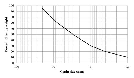
Fig. 4. Grain size distribution of well-graded sand
