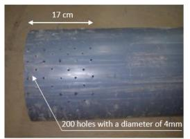
Fig. 2. Perforated polyethylene pipe
