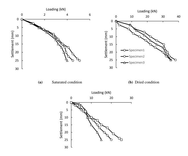
(c) Partially saturated condition Fig. 11. Load-settlement behavior of CLM column (column alone loaded) specimens
