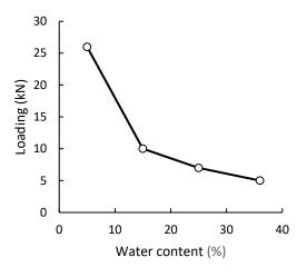
Fig. 12. The effect of percentage of lime mortar moisture on strength of CLM column specimens
