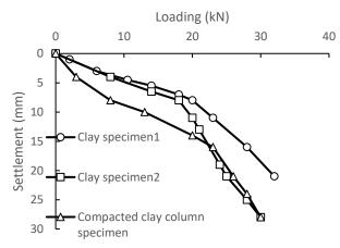
Fig. 16. Load-settlement behavior of compacted clay column (column alone loaded) specimen and clay specimens
