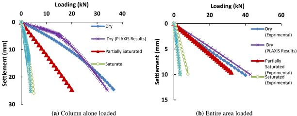
Fig. 19. Load-settlement curves for CLM column specimens
