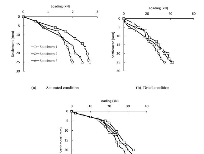
(c) Partially saturated condition Fig. 9. Load-settlement behavior of untreated layered soils
