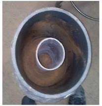
(a) Compacted soil layer and pipe on the second layer
