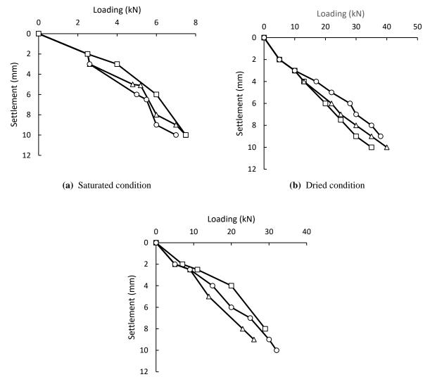
(c) Partially saturated condition Fig. 13. Load-settlement behavior of CLM column specimen (entire area loaded)
