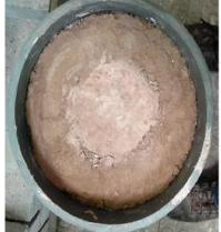
(c) Placing lime mortar in the central part of the mold
