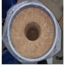
(b) Removing pipe after completing the soil compactionFig. 5. Preparing CLM column specimens
