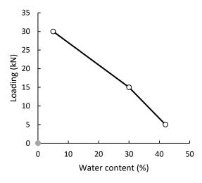
Fig. 10. The effect of percentage of moisture on clayey specimen's strength
