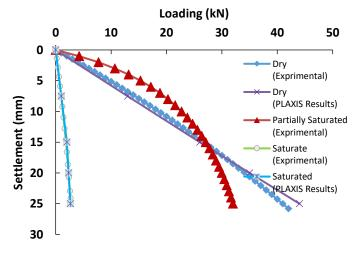
Fig. 18. Load-settlement curves for clay specimens
