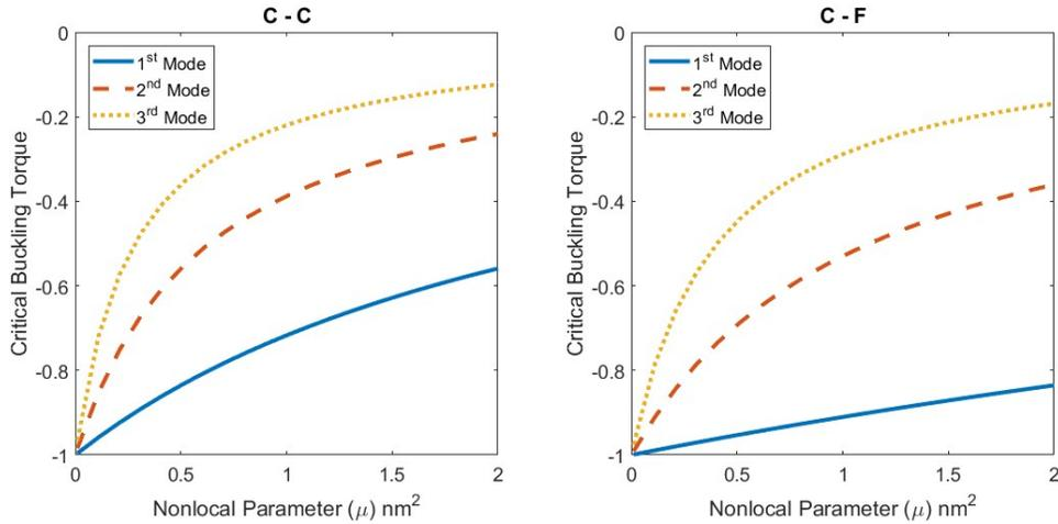
Figure 9. Variation of Critical Buckling Torque with Nonlocal Parameter ( $L=5\text{nm}$ )
