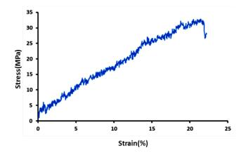
Fig. 7- Stress-strain curves of P(HEMA-b-NIPAAm-b-CL)/PANI electrospun nanofibers.
