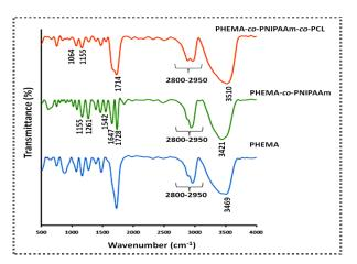
Fig. 2- FT-IR spectra of PHEMA, P(HEMA-b-NIPAAm), and P(HEMA-b-NIPAAm-b-CL).
