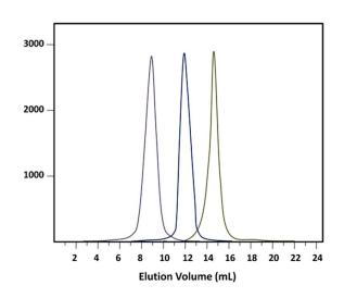
Fig. 4- GPC traces of PHEMA (green), P(HEMA-b-NIPAAm) (dark blue), and P(HEMA-b-NIPAAm-b-CL) (purple) in DMF as eluent.
