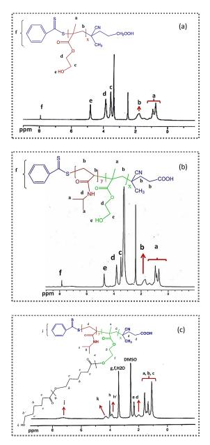
Fig. 3- <sup>1</sup>HNMR spectra of PHEMA (a), P(HEMA-*b*-NIPAAm) (b), and P(HEMA-b-NIPAAm-*b*-CL) (c).
