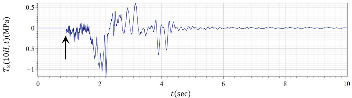
Fig. 10. Time-history of  $T_2(10H, t)$  in case 2. The arrow indicates the arrival of the first wavefront at  $t = 0.9$  sec
