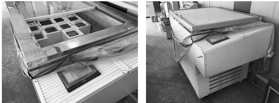
Fig. 5. Apparatus for simulating freeze-thaw cycles
