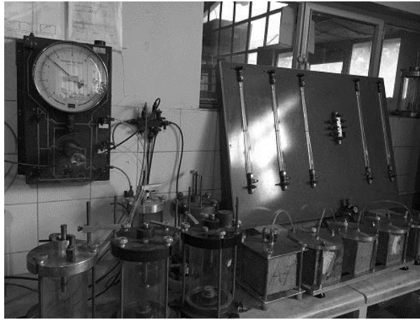
Fig. 3. Apparatus for measuring water depth of penetration
