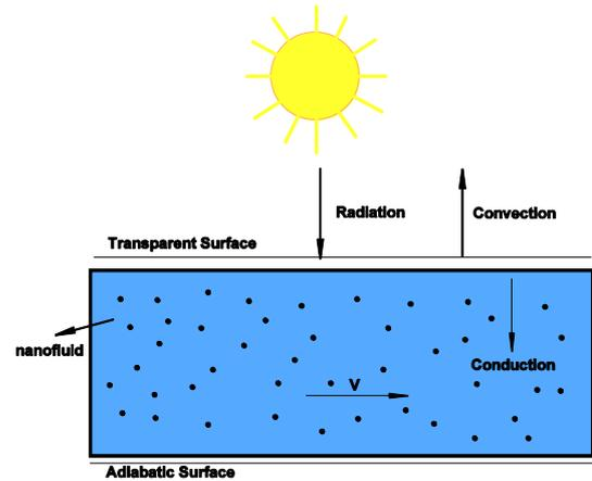
Figure 1. Schematic of the nanofluid-based direct absorption solar collector.
