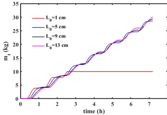
Figure 6. Effect of initial water depth on total water production during seven days of continuous process
