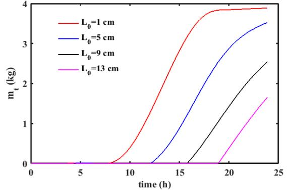
Figure 5. Effect of initial water depth on total water production during 24h
