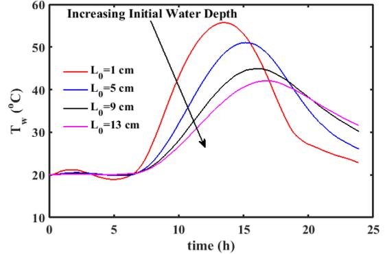
Figure 4. Effect of initial water depth on water temperature during 24h
