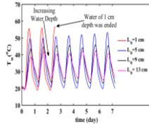
Figure 9. Effect of initial water depth on water temperature in seven days continuous cyclic process in Shiraz
