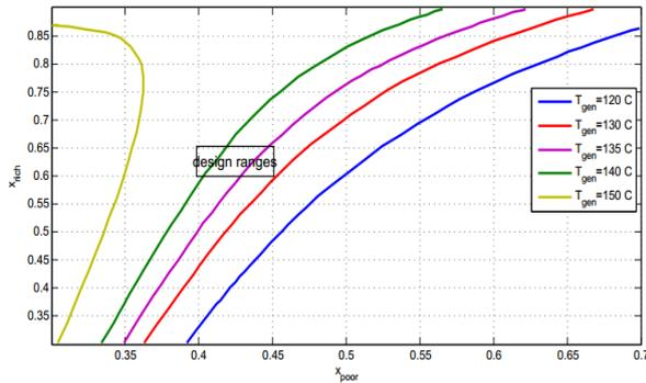
Figure 8. generator temperature contour vs concentrations in appropriate COP range
