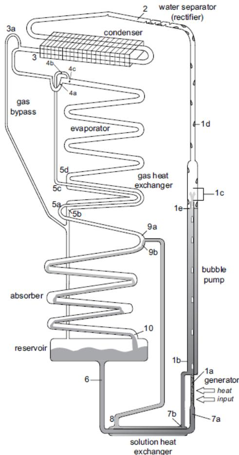
Figure 1. schematic of parts and key points of diffusion absorption cycle [7]
