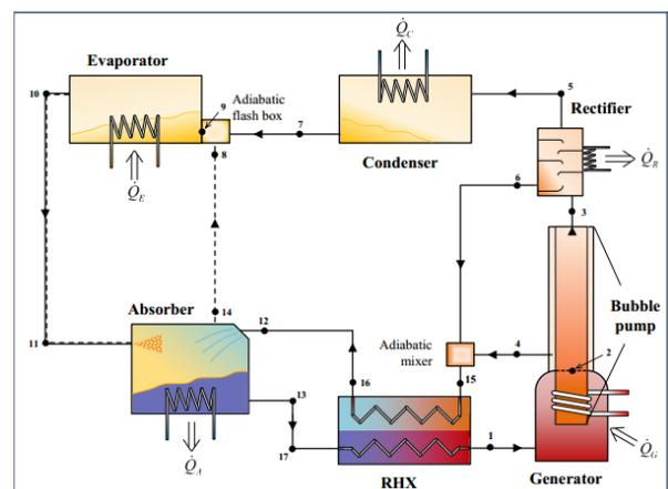
Figure 2. The solar diffusion absorption cycle in this study [11]
