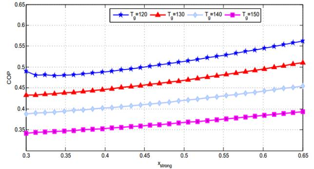
Figure 6. DAR performance with varying generator temperature and concentration of strong ammonia solution
