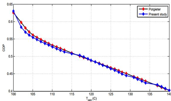
Figure 4. Comparison value of COP generator temperature in two studies
