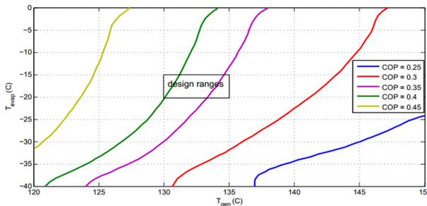
Figure 9. COP contour vs outstanding cycle temperature in appropriate generator temperature
