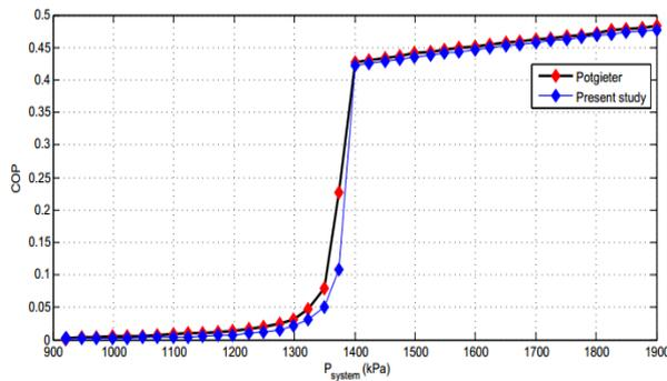
Figure 3. Comparison value of COP against pressure cycle in two studies
