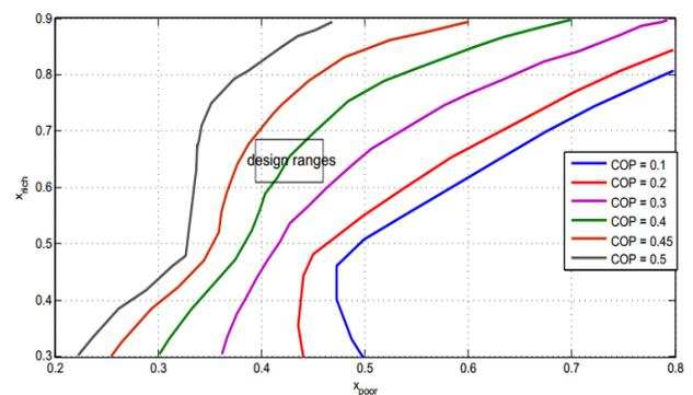
Figure 7. COP contour vs rich and poor solution concentration
