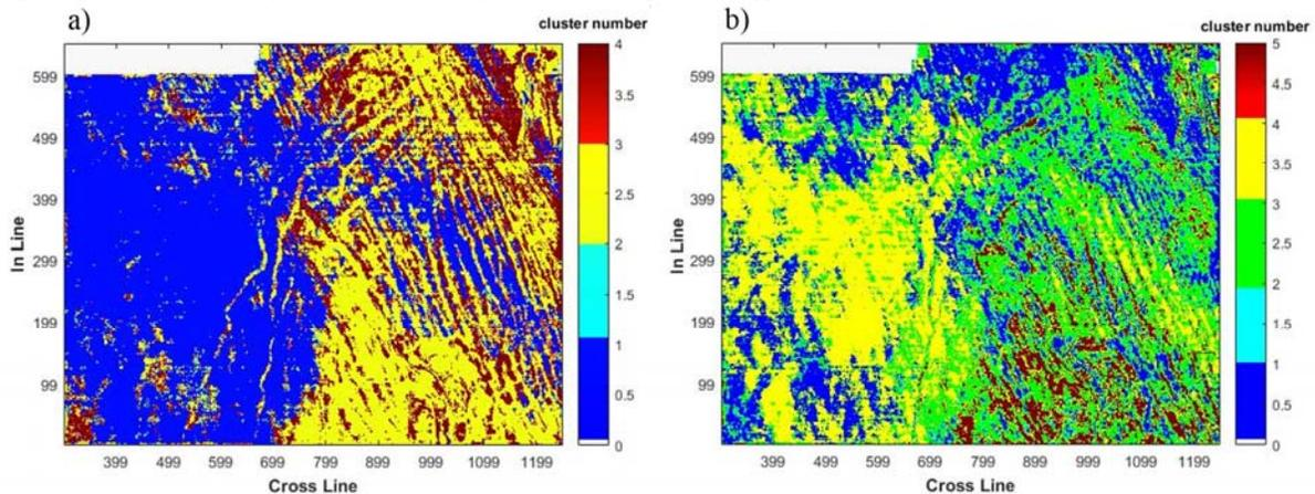
Figure 4. seismic facies analysis result obtained by GK clustering method applied on a) seismic attributes set and b) KPCA attributes.
