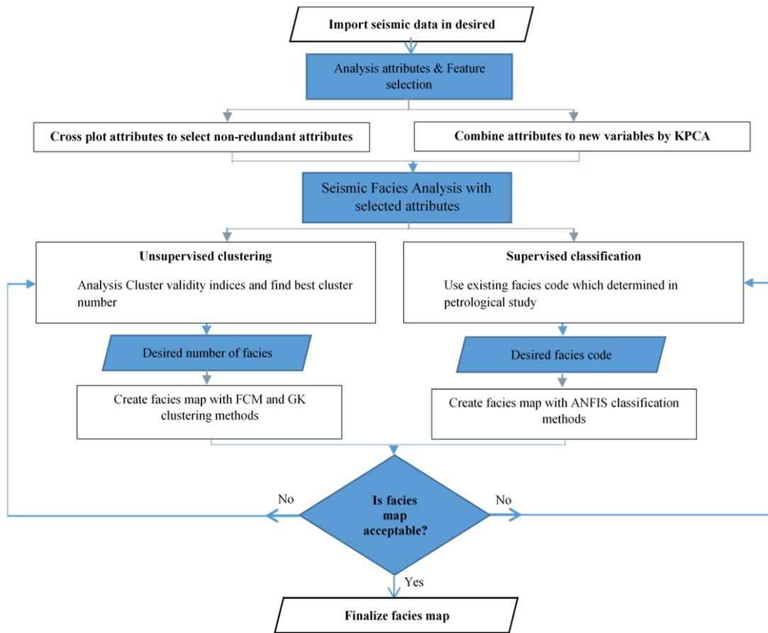
Figure 1. The workflow of seismic facies analysis
