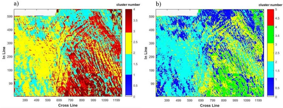
Figure 3. seismic facies analysis result obtained by FCM clustering method applied on a) seismic attributes set and b) KPCA attributes.
