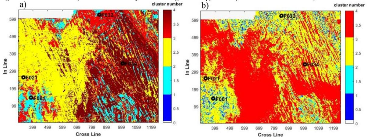
Figure 5. Seismic facies analysis result obtained by ANFIS clustering method applied on a) seismic attributes set and b) KPCA attributes. The well locations are remarked on figures.
