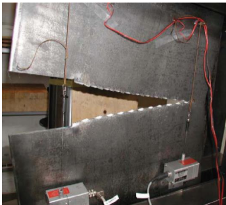
Fig. 6. Comparing of experimental with FE modeling; crack opening
