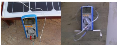
Figure 7: measurement of the ambient temperature around the module
