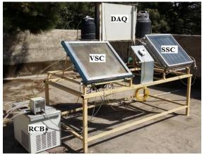
Figure 6. Test setups for the collector prototypes
