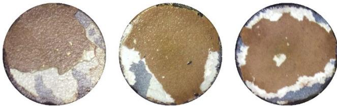
Fig. 8 Samples with CSZ coating after damage
