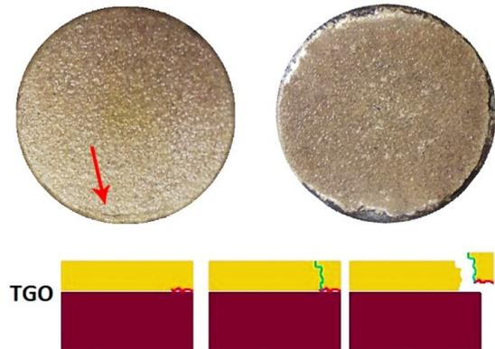
Fig. 4 (a) Starting and growth of damage in the YSZ class and (b) Schematic representation of location and how damage occurred
