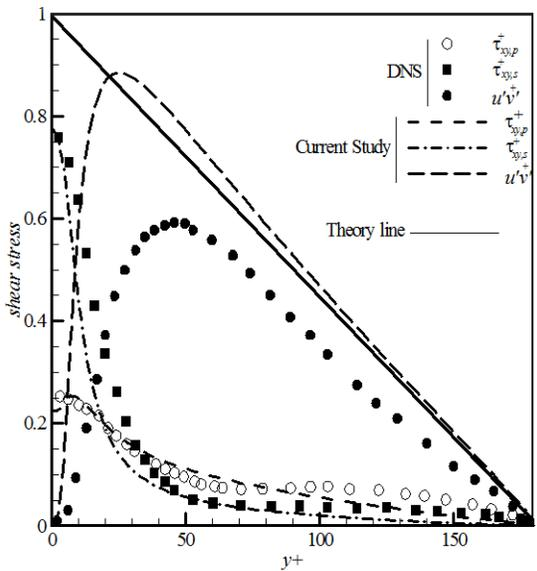
Figure 8- Normalized wall shear stress profile for DNS data [3] and current study in case D1 (a) and D4 (a)
