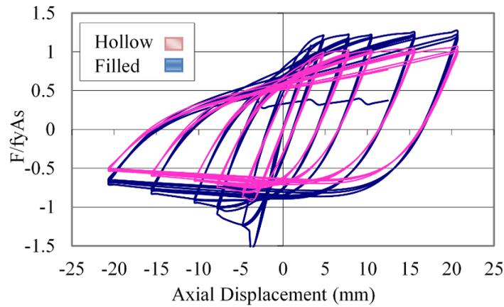
Fig. 6. Comparison of hollow and concrete filled in specimen 12 ( $l = 39.1$ )
