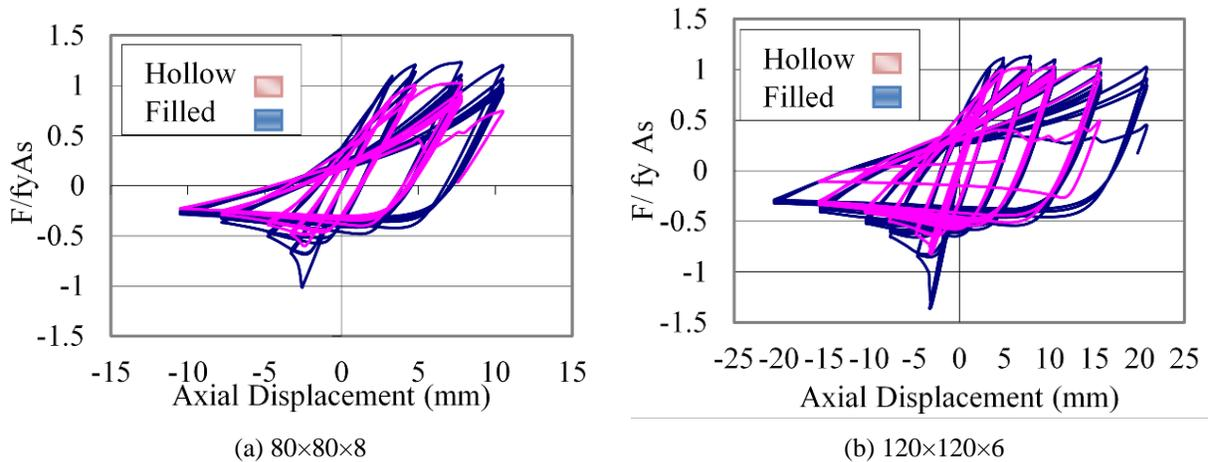
**Fig. 4.** Comparison of hollow section and concrete filled specimens
