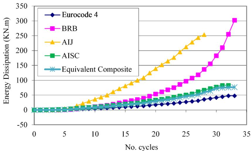
**Fig. 9.** Energy absorbed in each cycle for specimen designed by different codes
