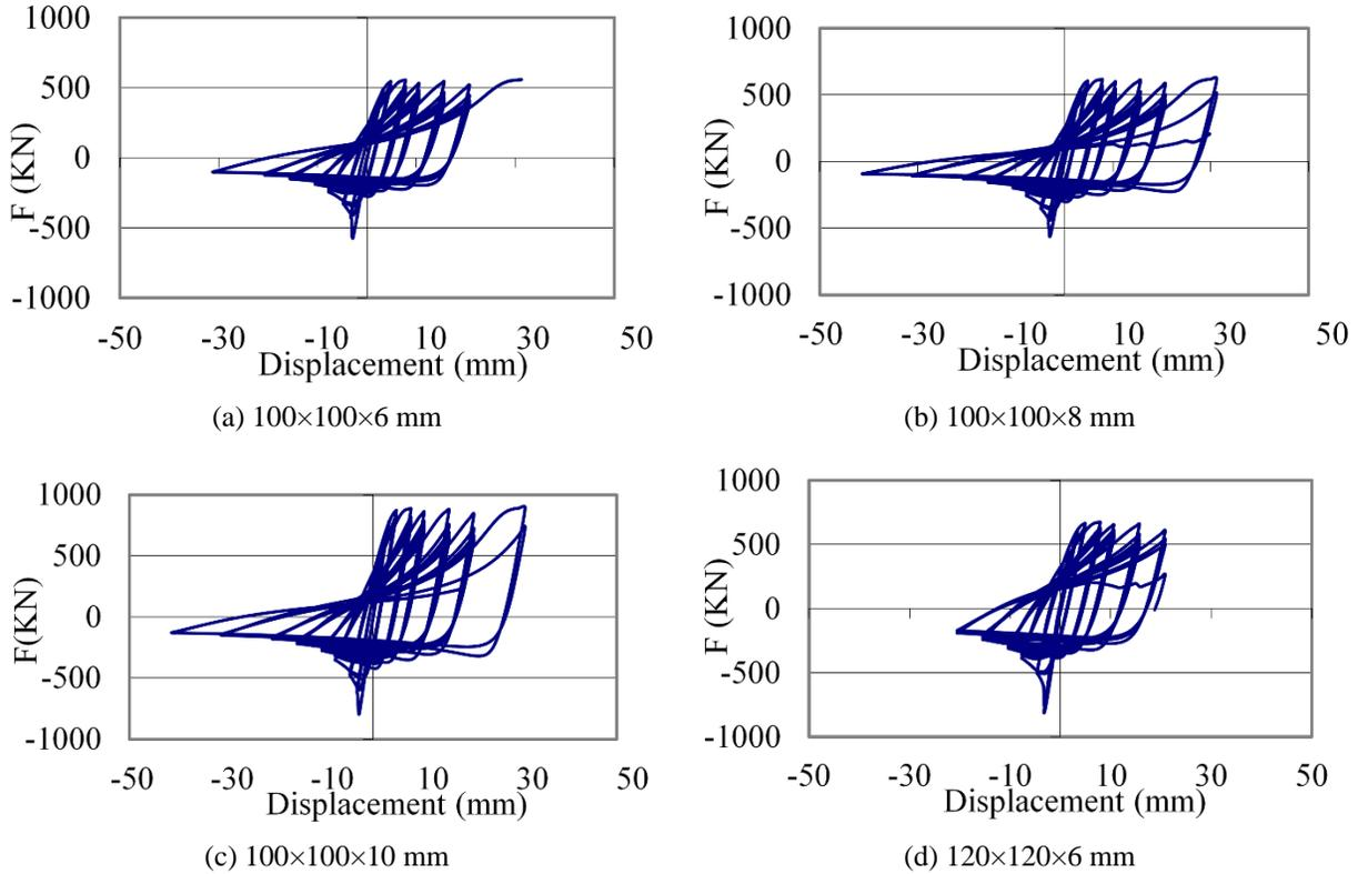
**Fig. 3.** The numerical load-displacement response of specimens
