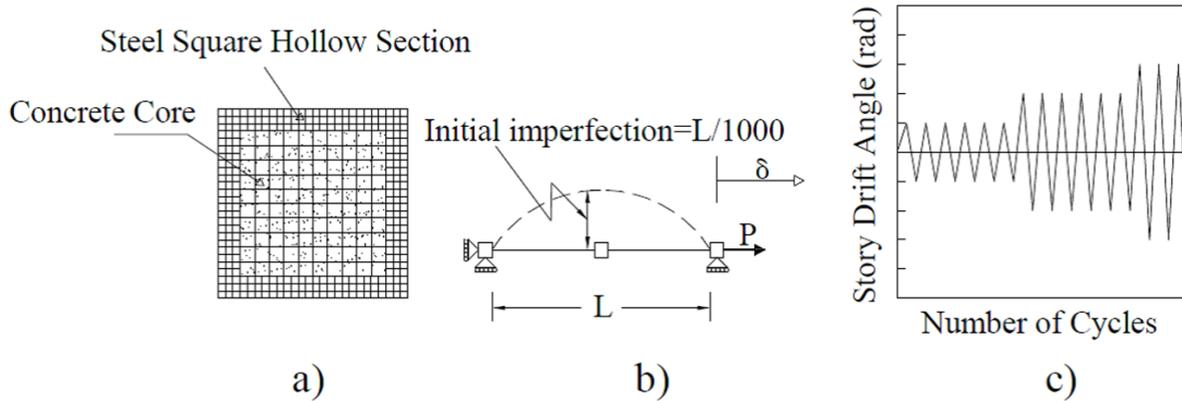
Fig. 1. Geometry and loading for numerical study; a) Composite section; b) Loading; c) Displacement history
