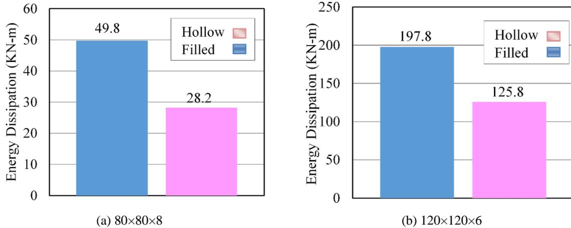
Fig. 5. Comparison of energy dissipation of hollow section and concrete filled specimens
