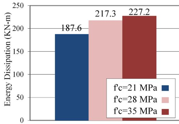
(a) Concrete with different compressive strength and A36 steel
