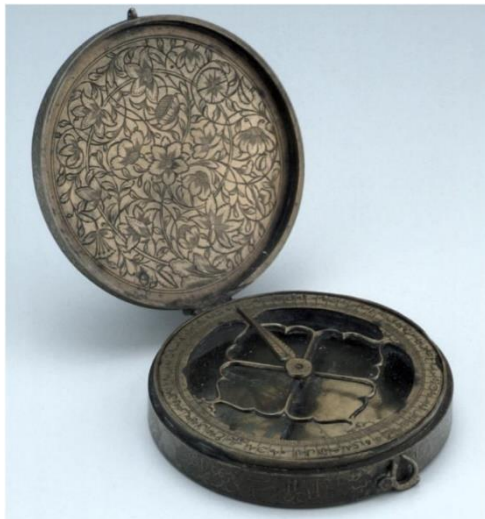
Fig. 9: A brass qibla-indicator of the kind of “ āy īni-yi gītī-numā ”. The distinctive verse engraved on the rim is barely legible. (Museum of the History of Science, Oxford)
